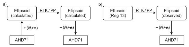
Figure 1: GNSS height transfer methodology using RTK or post processing (PP) in the past (a) and using CORS (b).
