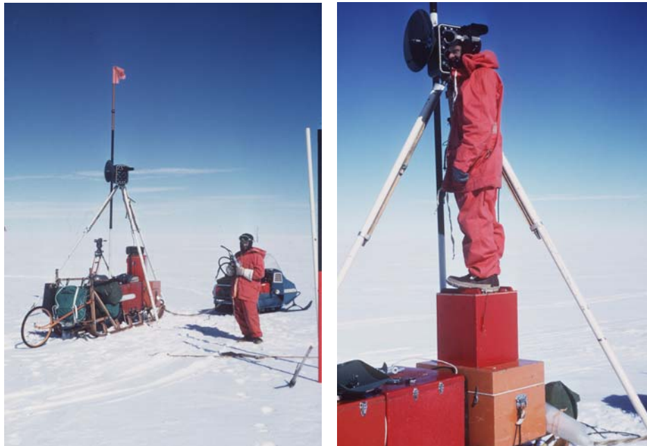
Fig. 3: Tellurometer set-up at a 'Corry' pole in 1970. The sledge-wheel is visible on the left. Photographs by Max Corry (left) and Norman Linton-Smith (right), Australian Government Antarctic Division © Commonwealth of Australia.
