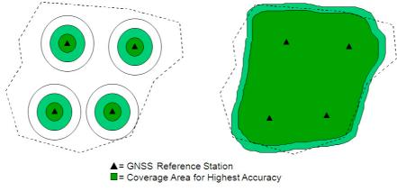
Figure 2: RTK vs. NRTK coverage.
