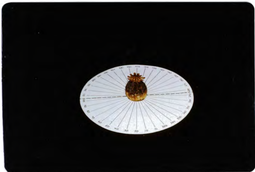
Plate 17. The compass ring apparatus used to measure the "central focus" and "angular range" of fungal colonisation. The row orientation of field plots is represented by the thick black broken line and the capsule is placed in the centre of the ring as shown.
