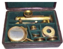
Figure 31: Ellis aquatic microscope c. 1775.
