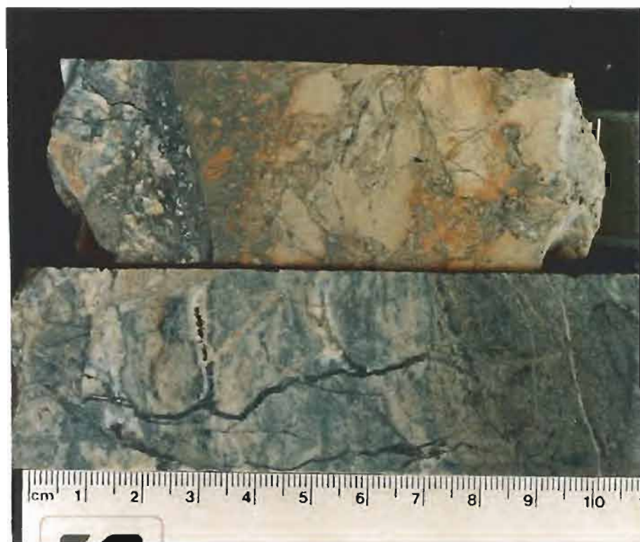
Fig. 5.12 Brecciated and massive siderite-pyrite rock from the upper intersection of the lower mineralized horizon in DDR GCA. Note the distinct massive siderite-pyrite intersection. The pyrite in these samples formed by the replacement of magnetite.
