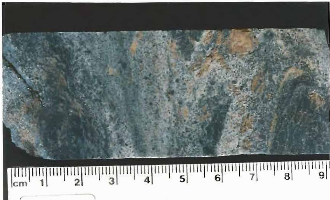
Fig. 5.10 Disrupted magnetite-barite-quartz-garnet (68263) from the middle intersection of the lower mineralized horizon of DDH GCB. The dirty yellow brown mineral is andradite garnet and the white zones are a mixture of barite and quartz.
