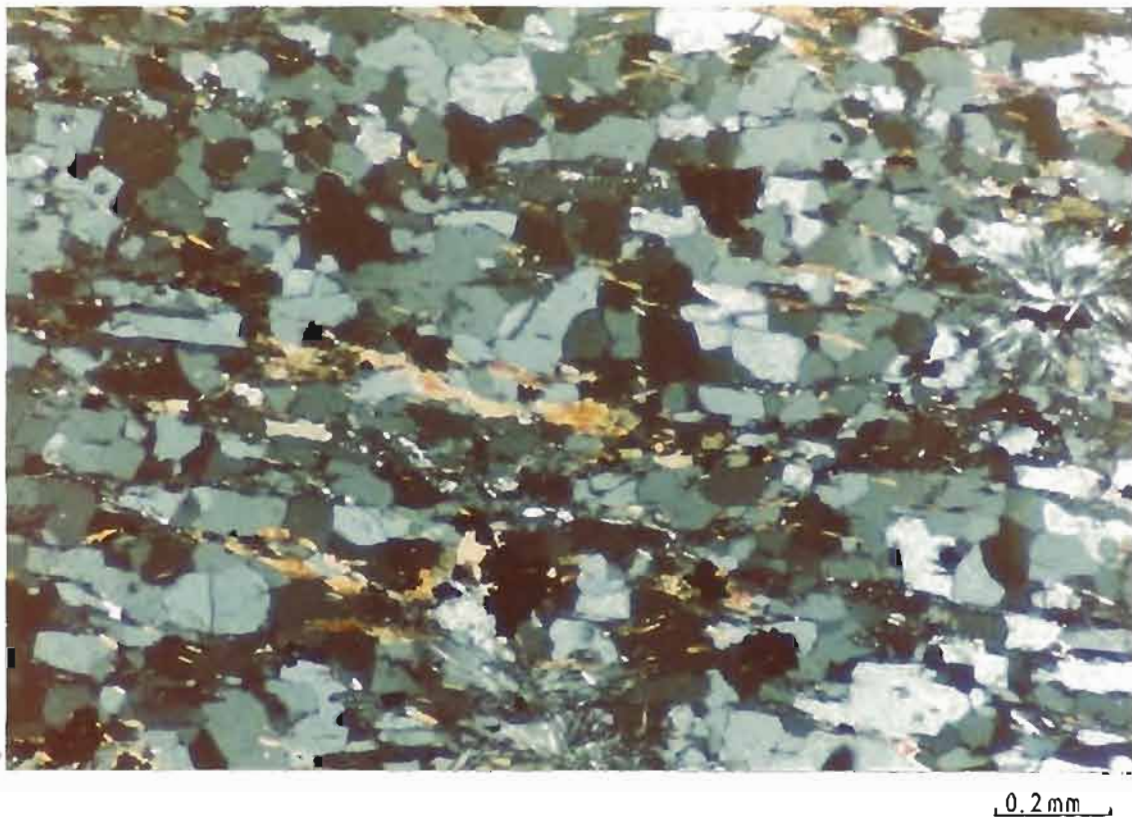
Fig. 4.4 Highly annealed granoblastic quartz-biotite-sillimanite hornfels typical of the hornblende hornfels facies. Sillimanite in this sample forms radiating clusters of fine grained, low birefringent, acicular grains. Polarized light photomicrograph.
