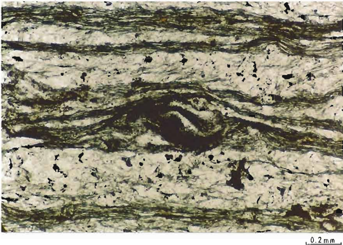
Fig. 4.3 Quartz-muscovite-albite-epidote-magnetite schist. Muscovite defines a crenulation cleavage consistent in orientation and style to the second phase cleavage. Albite porphyroblast (centre) has sigmoidal intrusion train defined by magnetite. Plane light photomicrograph.
