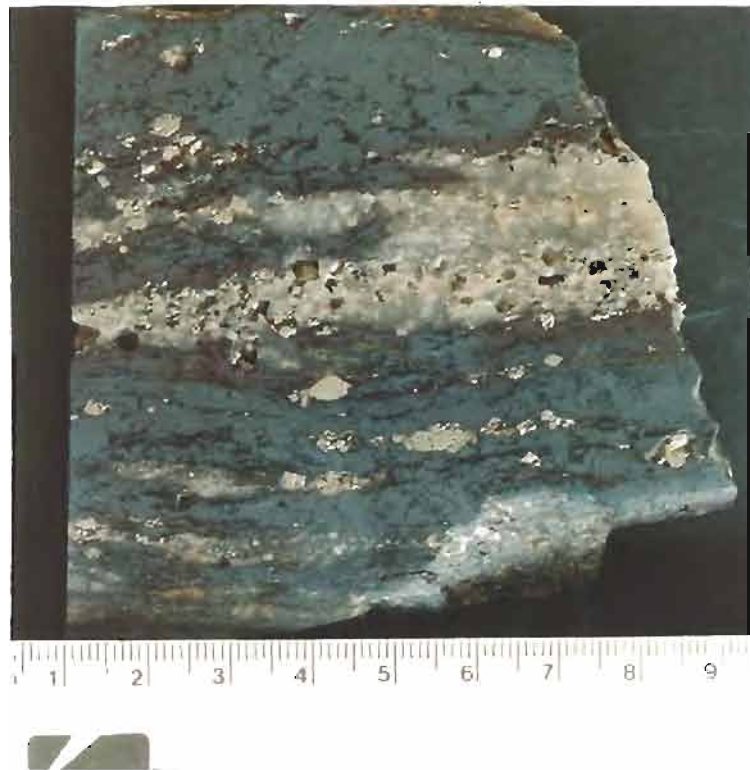
Fig. 5.4 Banded hematite-quartz rock (68273) with coarse grained, subhedral pyrite grains in both quartz and hematite layers. Sample from surface outcrop.
