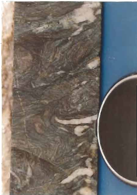
Fig. 5.4 Banded hematite-quartz rock (68273) with coarse grained, subhedral pyrite grains in both quartz and hematite layers. Sample from surface outcrop.
