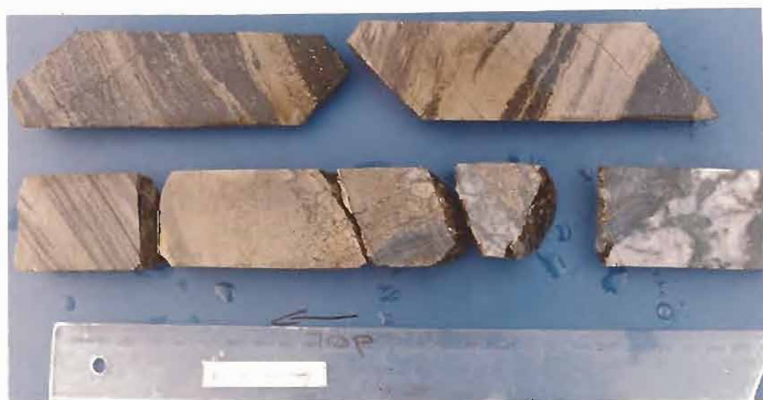
Fig. 5.9 A pyrite-rich intersection of the lower mineralized horizon in DDH GC3. The footwall is in the lower right hand corner and the hangingwall in the upper left hand corner. Zoning from the footwall upwards is: disrupted quartz veining, massive clastic (brecciated) pyrite, massive fine grained pyrite, banded magnetite pyrite, and finally, banded pyrite hornfels.
