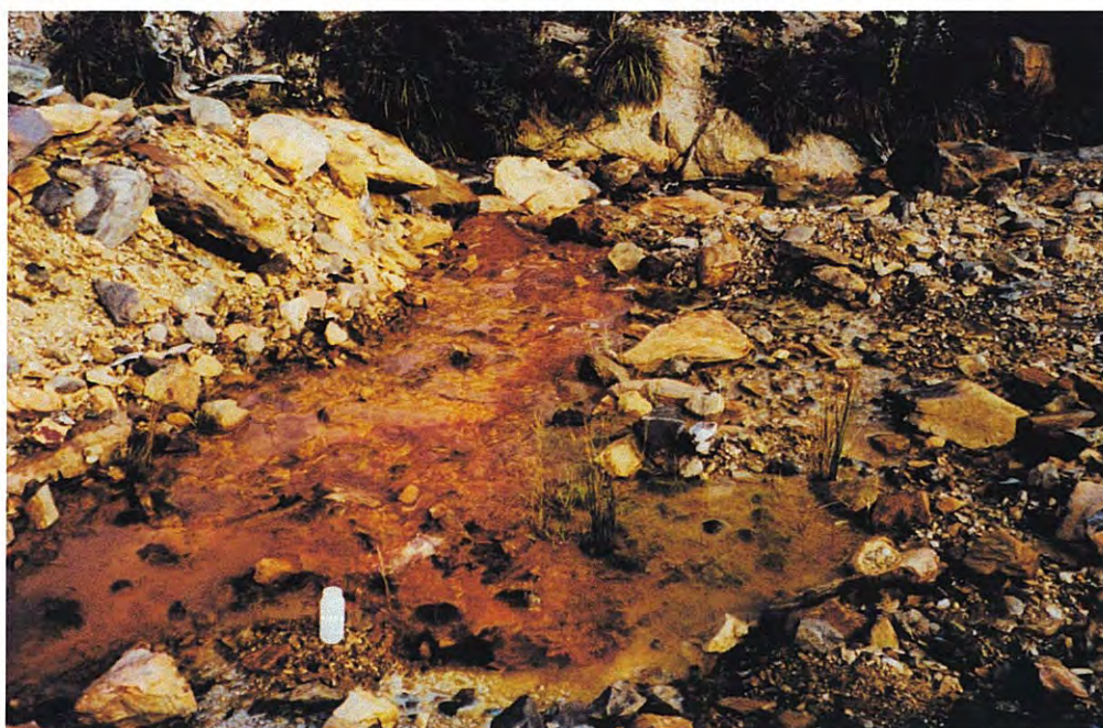
Plate 4.2 (A) Precipitates located at the base of the waste rock dump at Site F ; (B) Precipitates deposited outside the mouth of the Adit at Site C. The drainage from the adit flows directly into Bakers Creek.
