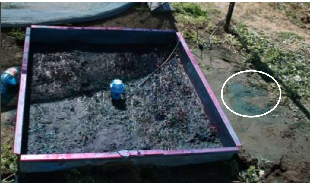
Figure 4.4-2 Site D, wet treatment. Lateral movement of dye tracer through the A1 horizon resulting in the patch of dye stained soil to the right of the application area (white ring).
