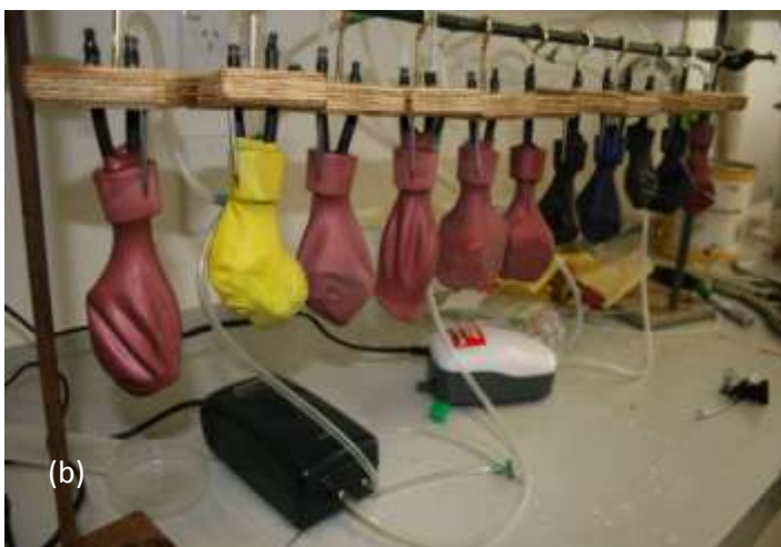
Figure 6.2-3 Balloon technique for determination of SSCC. (a) Measurement of soil clod volume by Archimedes principle. (b) Drying multiple soil clods with aquarium air pumps. (c) Air evacuated from soil clod, photographed following immersion to determine volume.
