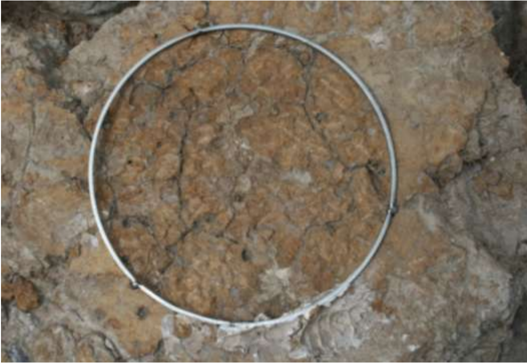
Figure 6.2-9 Picked back surface of B21 horizon , dry treatment, showing soil cracks, sand infills and red headed cockchafer beetle burrows (1 cm diameter 1 cm deep cylindrical holes).
