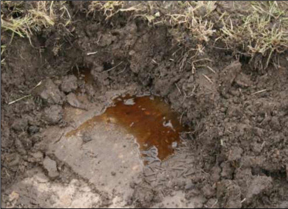
Figure 4.4-1 Site B, wet treatment. Subsurface lateral flow at A1 / A2 boundary. Flow may have been induced by compaction resulting from walking around the site.
