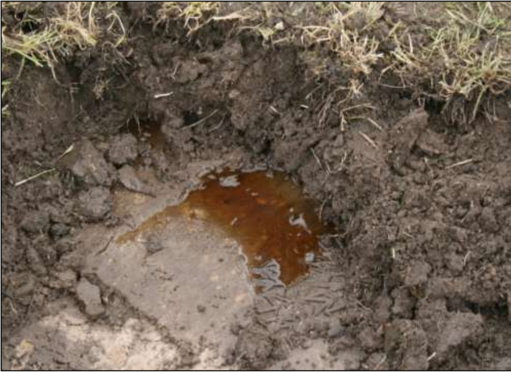
Figure 6.3-13 Site B, wet treatment. Subsurface lateral flow at A1 / A2 boundary.
