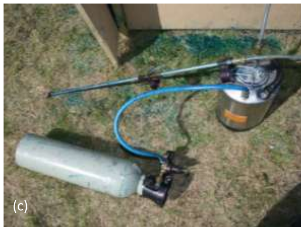
Figure 4.2-1 Dye application techniques: (a) Spray chamber used with hand held sprayer, note EnviroSCAN probe and localised ponding, (b) Rotating disk rainfall simulator used for dye application in the dry treatments at site A, B and C, (c) Hand held pressure sprayer used in all wet treatments, and the dry treatment at site D, (d) Calibration of the rainfall simulator.
