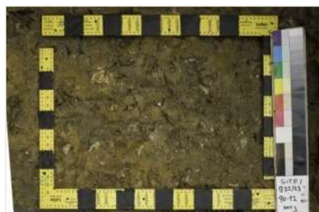
Figure 4.3-4 Site A, dry treatment. Horizontal excavation at 35 cm - 92 cm depth. First column - excavation depth and % of dye stained soil. Second column- dye stained soil. Third column - binary image of dye staining.
