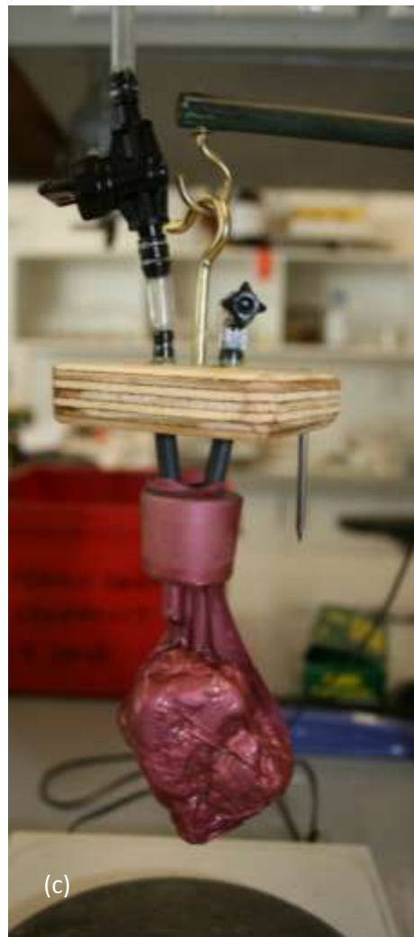
Figure 6.2-3 Balloon technique for determination of SSCC. (a) Measurement of soil clod volume by Archimedes principle. (b) Drying multiple soil clods with aquarium air pumps. (c) Air evacuated from soil clod, photographed following immersion to determine volume.
