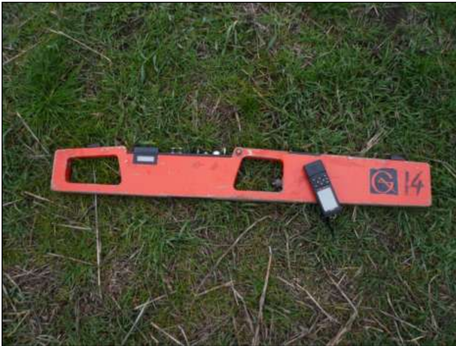
Figure 3.1-2 Equipment used for EMI survey, Geonics EMI38, ad Garmin 12 XI GPS
