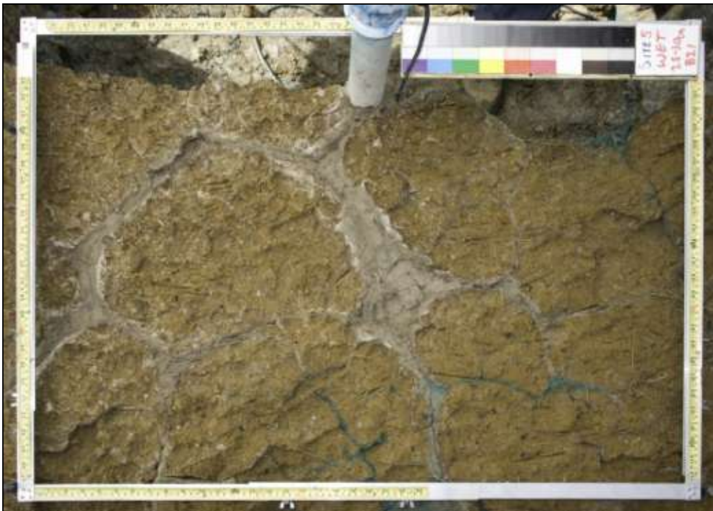
Figure 4.3-37 Lack of dye staining in upper B21 and sand infills at site B- wet treatment 0.8 % dye stained.
