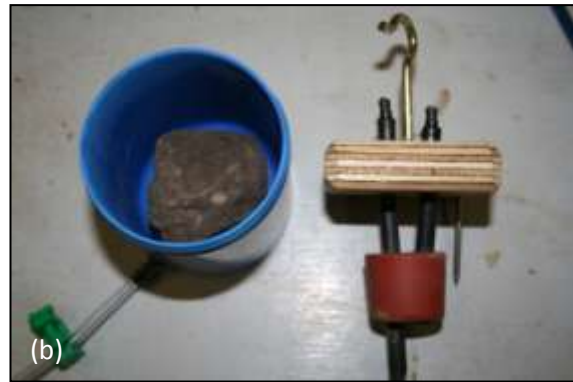
Figure 6.2-2 Preparation of samples for balloon determination of SSCC, (a) Wetting up soil clods using Haines apparatus, (b) Suction vial for getting soil clods into the balloons, and setup apparatus showing inflow and outflow tubes.
