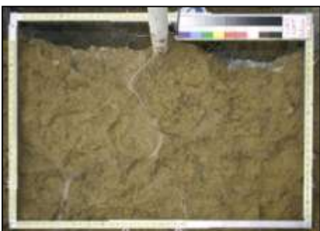
Figure 4.3-14 Site B. Wet treatment. Horizontal excavation 18cm - 45 cm depth. First column - excavation depth and % of dye stained soil. Second column- dye stained soil. Third column - binary image of dye staining.
