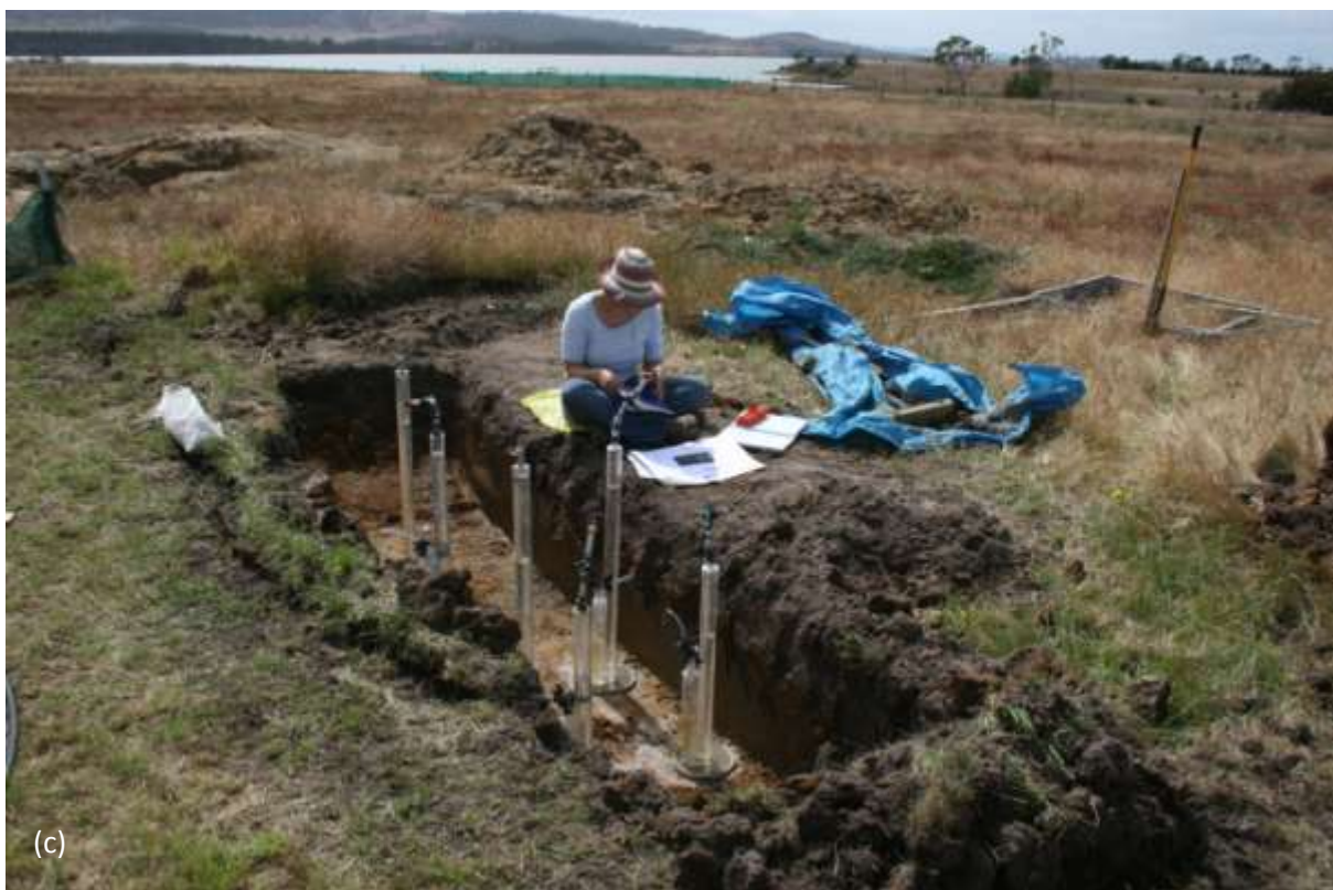
Figure 6.2-8 (a) Recently constructed tension infiltrometer with multiple tube bubble tower to enable rapid change in supply potential. Measurement of subsoil unsaturated hydraulic conductivity, (b) site C, and (c) site B.
