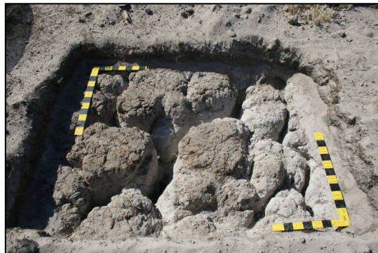
4) Site B. Extensive development of cracks and sand infills. Upper B2 had strong columnar structure.
