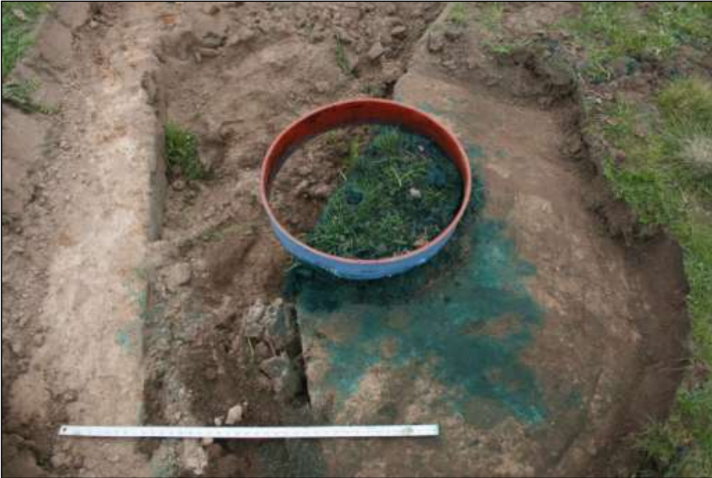
Figure 4.3-48 Trial application of 50 mm dye tracer at site A, wet treatment, showing considerable lateral movement of the dye tracer above the B21 and A2 horizon.
