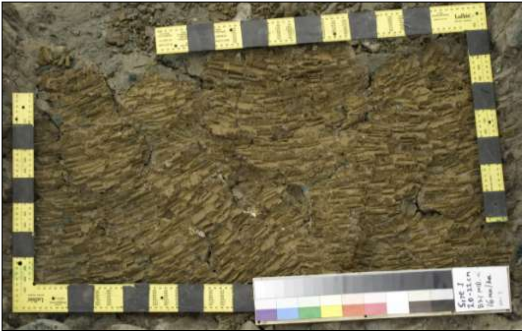
Figure 4.3-36 Site A, dry treatment. Horizontal excavation revealed that bypass flow occurred in only 0.33 % of the B21 horizon.
