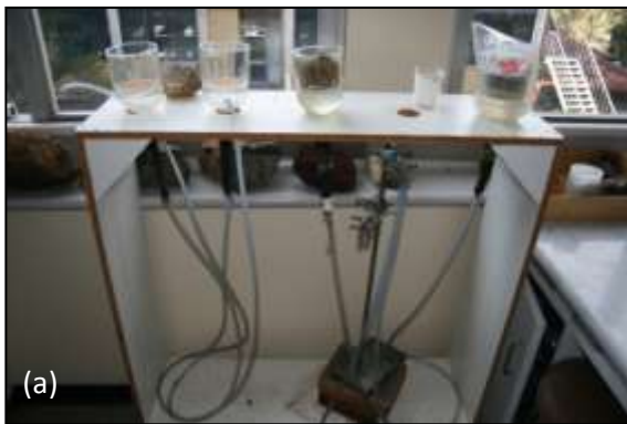
Figure 6.2-2 Preparation of samples for balloon determination of SSCC, (a) Wetting up soil clods using Haines apparatus, (b) Suction vial for getting soil clods into the balloons, and setup apparatus showing inflow and outflow tubes.
