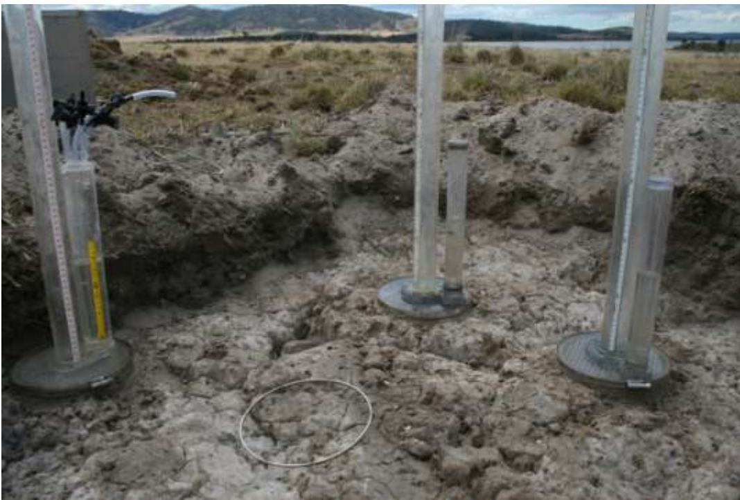
Figure 6.2-10 Measurement of hydraulic conductivity on the upper surface of the B21 horizon at site C.
