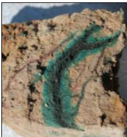
Figure 4.3-45 Dye staining along pre-clearing root holes, site B.
