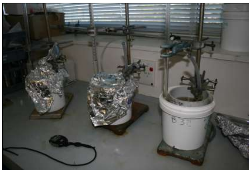
Figure 6.2-5 Determination of saturated hydraulic conductivity using constant head approach on 100 mm diameter intact soil cores. Note foil to prevent evaporation on soils with slow flow rates.
