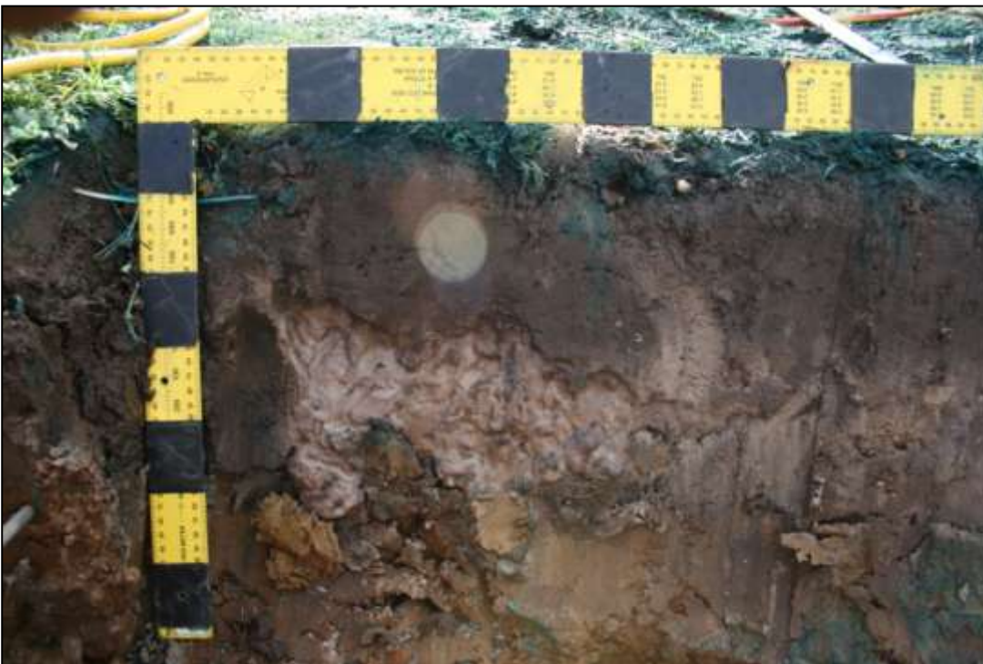
Figure 4.3-49 Site B, wet treatment. Saturation and lateral movement of the A2 horizon.
