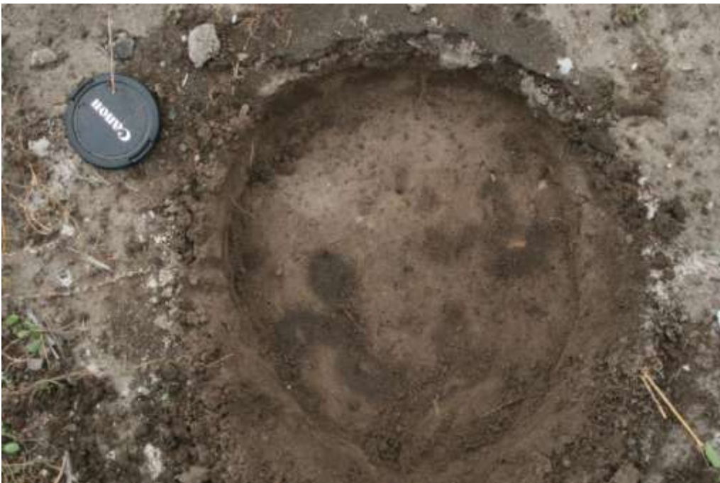
Figure 6.3-6 Development of finger flow beneath a tension infiltrometer during infiltration into soil at low antecedent soil moisture.
