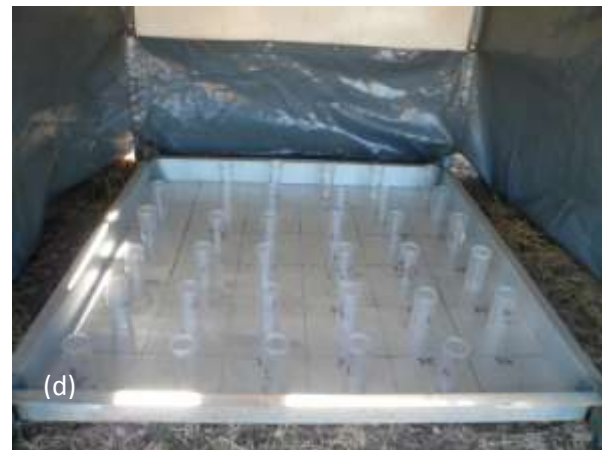
Figure 4.2-1 Dye application techniques: (a) Spray chamber used with hand held sprayer, note EnviroSCAN probe and localised ponding, (b) Rotating disk rainfall simulator used for dye application in the dry treatments at site A, B and C, (c) Hand held pressure sprayer used in all wet treatments, and the dry treatment at site D, (d) Calibration of the rainfall simulator.
