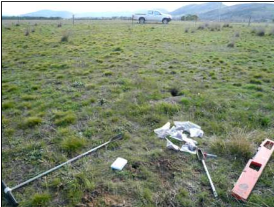
Figure 3.1-3 Equipment used in sample collection for calibration of EMI data, Far Dam paddock.
