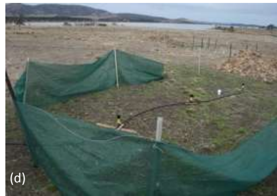
Figure 4.1-1 Establishment of soil water treatments: (a) Rainout shelter located at site D. (b) Irrigation supplied by 100 drippers in a 3 x 3 meter area. Water application was controlled by battery powered timers, supplied from two 44 gallon reservoirs. (c) Sprinklers at sites A, B and C were connected to S.E. irrigation scheme adjacent a stock drinking trough. (d) Sprinkler set up at site C, note shade cloth as a permeable wind fence and EnviroSCAN probe.
