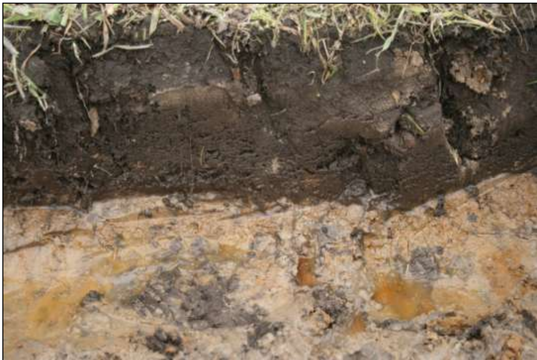
Figure 4.3-50 Saturation at the A1 / A2 boundary, site B wet treatment.
