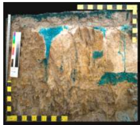
70 mins: Filling from below between clay columns and filling of smaller dead end pores in the B21 and B22 horizons. 30 cm sensor has yet to respond.
