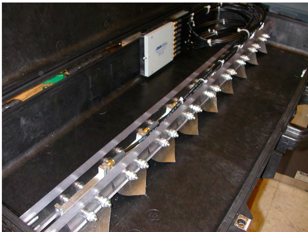
Figure A.6: Custom designed 8 - element TEM horn array for helicopter operation, shown here within radome (Pelican TM 1700 case).
