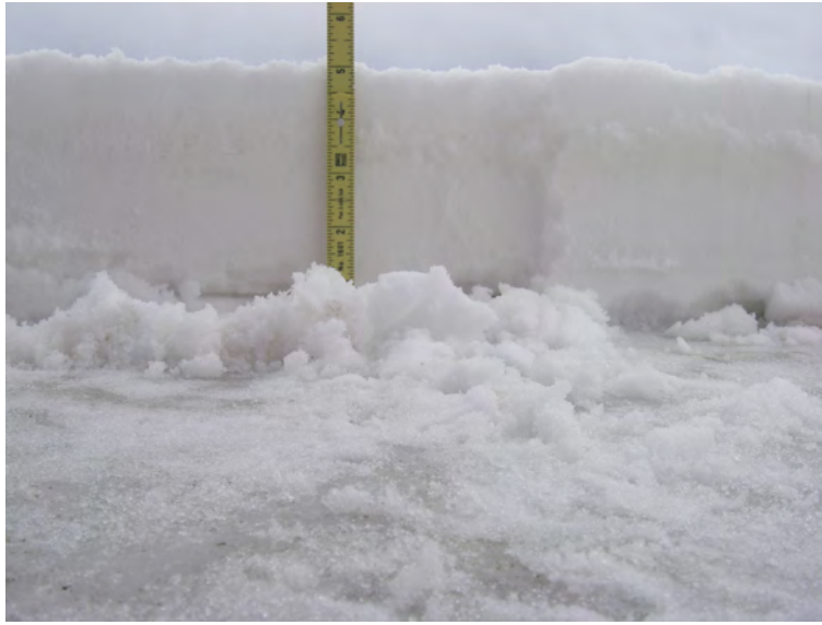
Figure 4.1: An example of a snow pit demonstrating the small vertical scale variability of surface height over decimetre scales. Various features of this snow pit were frequently observed in the sled-based study, such as the large depth hoar crystals and slush layer at the snow/ice interface. Additionally, a layer of dirt, probably blown from the Vestfold Hills appears about 35 mm above the ice surface.
