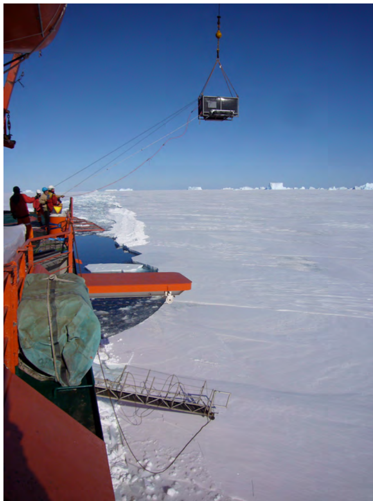
Figure 6.5: The radar inside a cage pallet and attached to the ship's crane for testing. Photo credit: J. Lieser. The radar antennas are secured to the bottom of the cage pallet.
