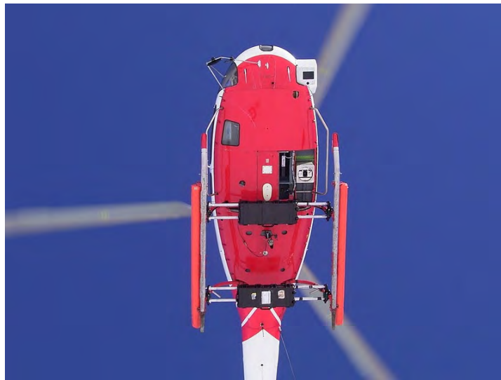
Figure 6.2: Photograph of the underside of the helicopter during flight. Courtesy of K.Newbery. The black rectangular window in the top right hand side of the helicopter is the laser scanner aperture, the two black rectangular boxes between the skids are the radar transmit and receive antennas, and the exposed box to the top right of the radar antennas is the camera lens.
