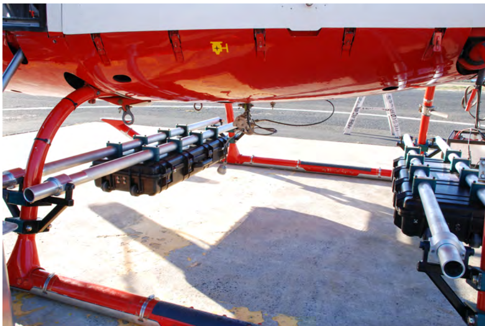
Figure A.7: Custom designed 8 - element TEM horn array in radome, attached between helicopter skids.
