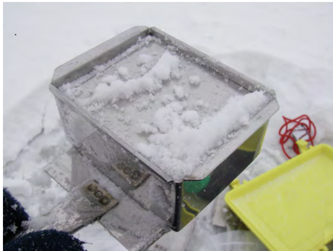
Figure 4.3: Snow density sampler tool, shown here filled with snow from a snow pit. Collecting a known volume of snow, allows the density of the weighted sample to be calculated.
