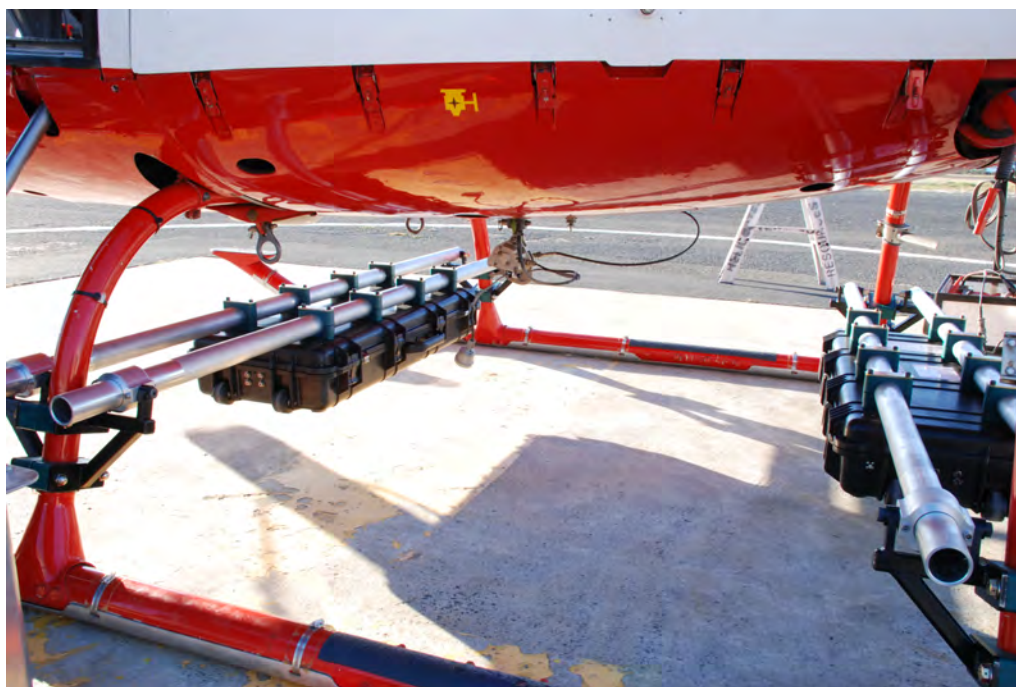
Figure D.4: Antennas in radomes, mounted between the skids of the Squirrel helicopter.
