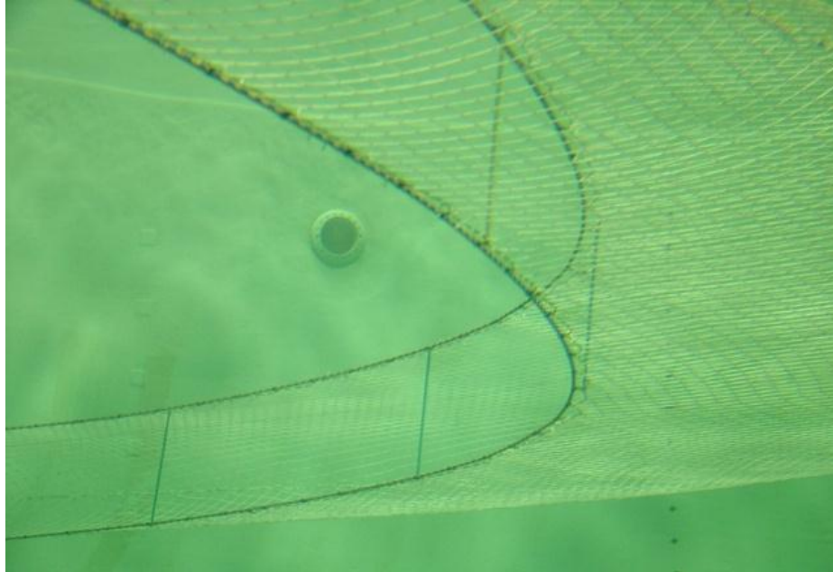
Fig. 4.4 Forepart of model-trawl during testing showing vertical struts fixing the vertical opening at the mouth.
