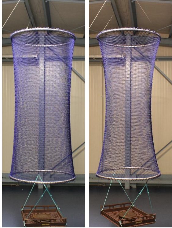
Fig. 3.7 Nylon samples in the longitudinal orientation attached to 1m diameter hoops with the horizontal mesh hanging coefficient of 0.32 and 0.44 (eq. 3.8 and Table 3.1). As seen, the distance between the hoops does not significantly change with hanging coefficient variation.
