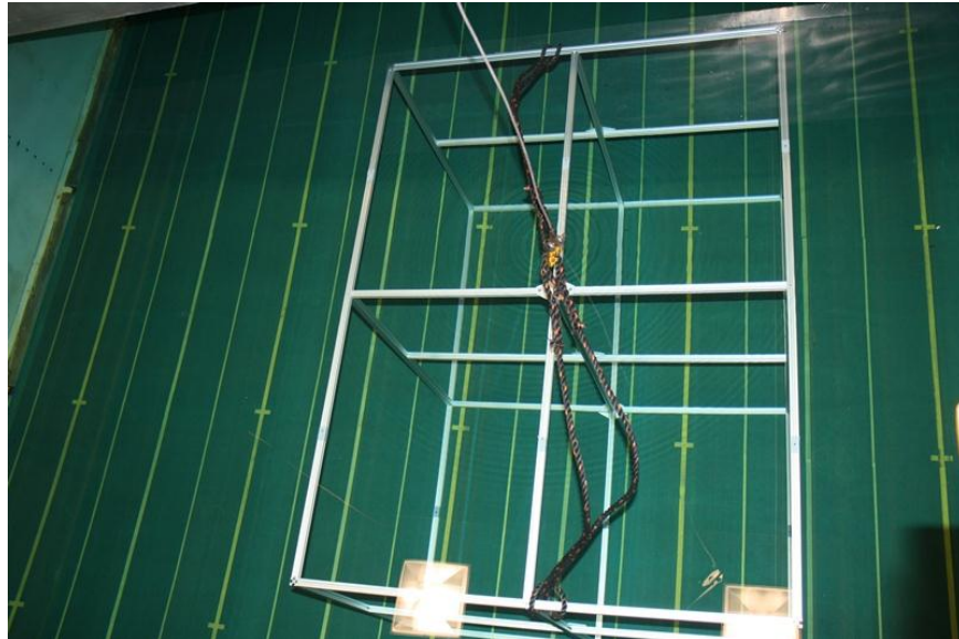
Fig. 4.7 A camera calibration frame - top view (in analysis, the image taken through the boat Perspex window was used to account distortions produced by the window).
