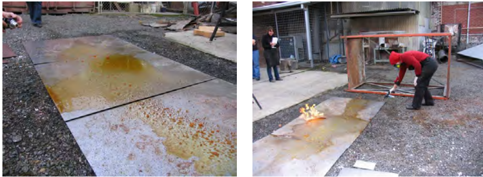
150. Photographs of throwing liquid rosin onto plates and setting alight.
