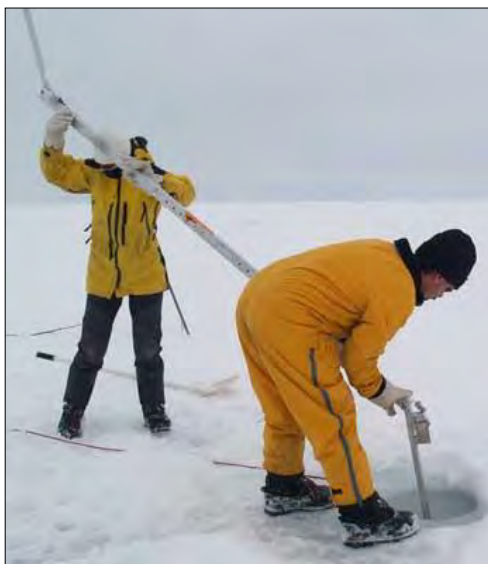
Figure 6.5: Feeding the 'Z' frame through the auger hole.
