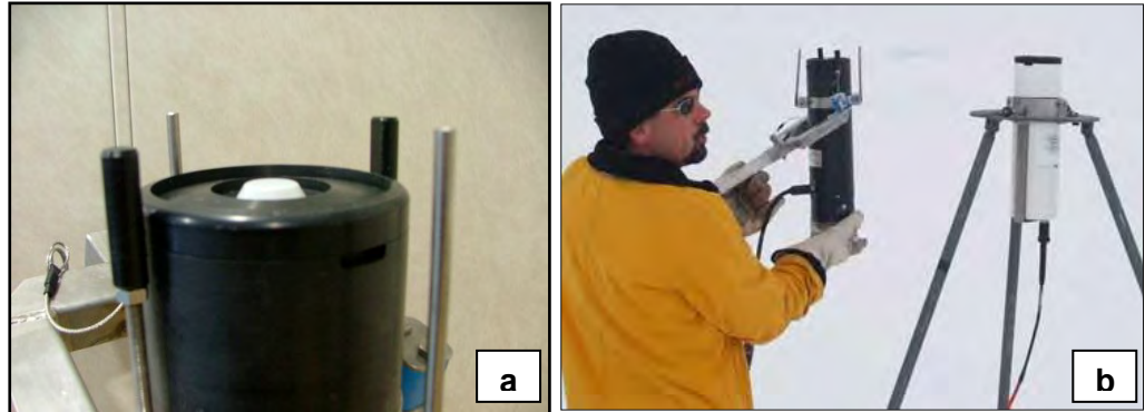
Figure 6.1: a. Top of PUV-2500 instrument and b. PUV-2500 held on the left and PUV-2510 fixed in tripod.
