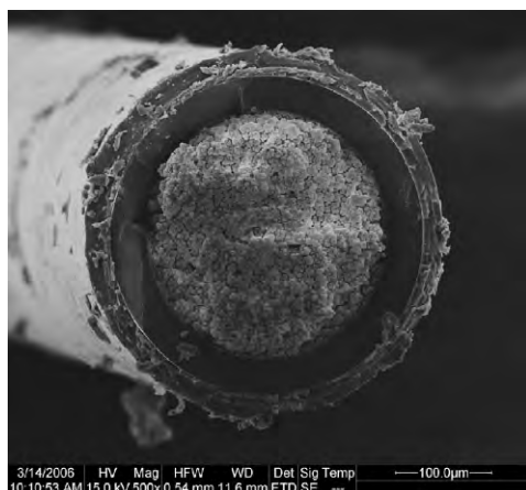
Figure 2. SEM of the monolith completely filling a 250 \mu\text{m} capillary.
