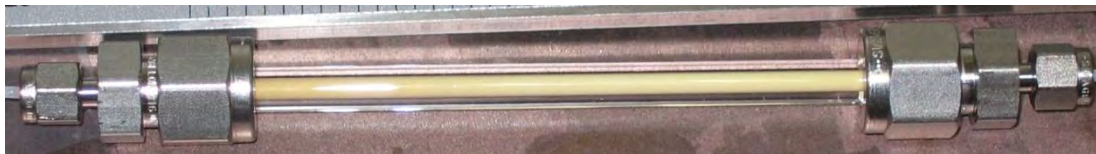
Figure 3.2 Poly(GMA- co -EDMA) in 2 mm ID column functionalised with 5-NH 2 phen.
