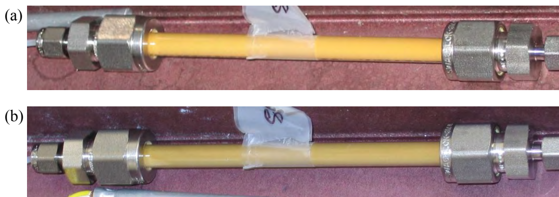
Figure 4.4 (a) LR3 reactor before reaction, (b) during the reaction.
