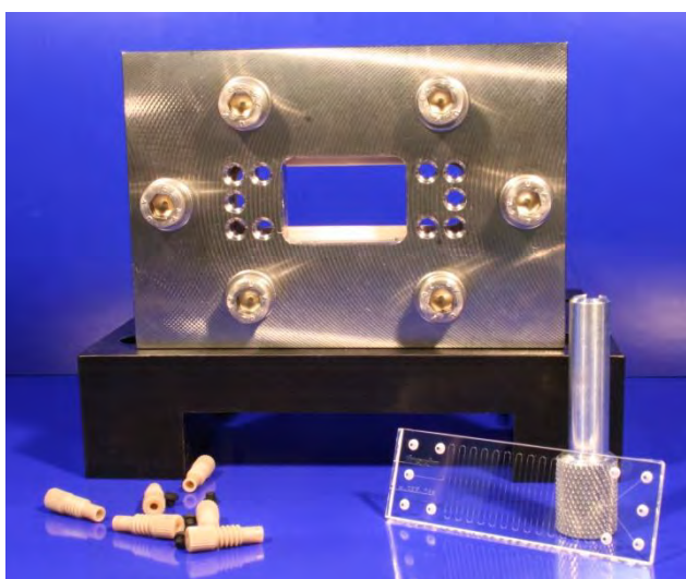
Figure 5.5 Micronit chip holder. Also visible is a glass microchip (bottom right) and fittings (bottom left). Image supplied by Micronit Microfluidics BV.
