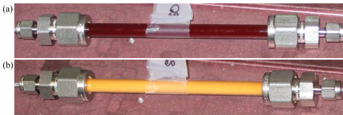
Figure 3.4 (a) During attachment of Me-im to poly(GMA-co-EDMA) monolith in a 4mm ID columns, (b) after the post-flush.
