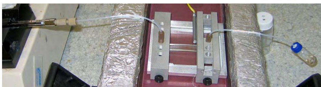
Figure 5.9 Complete microchip interface featuring a COC microreactor.
