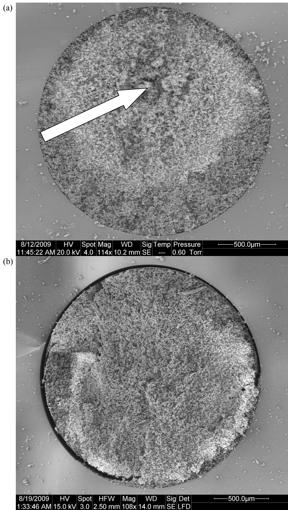
Figure 2.38(a) PPM in 2 mm ID column formed using UV-LED/BAPO with a 40 min exposure, (b) using Model 30/DMPAP.
