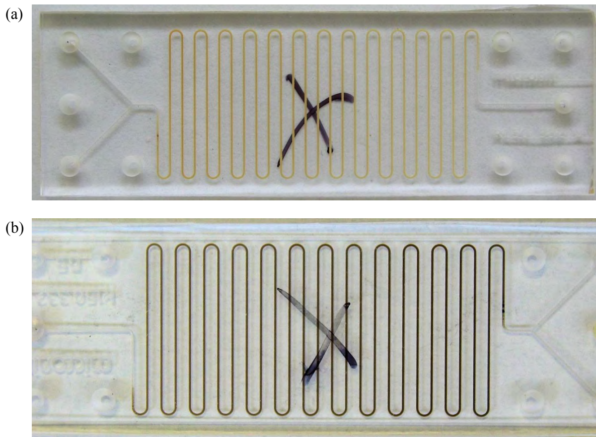
Figure 4.5 (a) Borosilicate microchip reactor before reaction, (b) and after.
