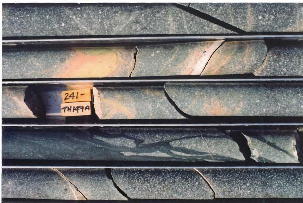
Figure 12b Semi pervasive and vein selvage epidote-albite alteration similar to that in dacite (above) but here occurring in post D2 deformation microdiorite dyke. Also shows multiple phases of mafic magma injection with feldspar porphyritic type intruded by finer grained, more mafic phase.
