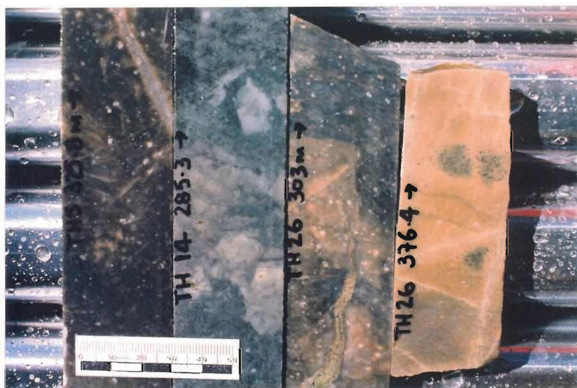
Figure 23. Four core specimens illustrating Group 6 siliceous "hanging wall" rhyolites; the specimen at right (TH26-376.4m) is typical of "Buff Rhyolite". These rocks are chemically similar to least altered footwall rhyolites and are interpreted to be structurally emplaced parts from the footwall. Some e.g. at left, superficially resemble felspar phyric dacite.
