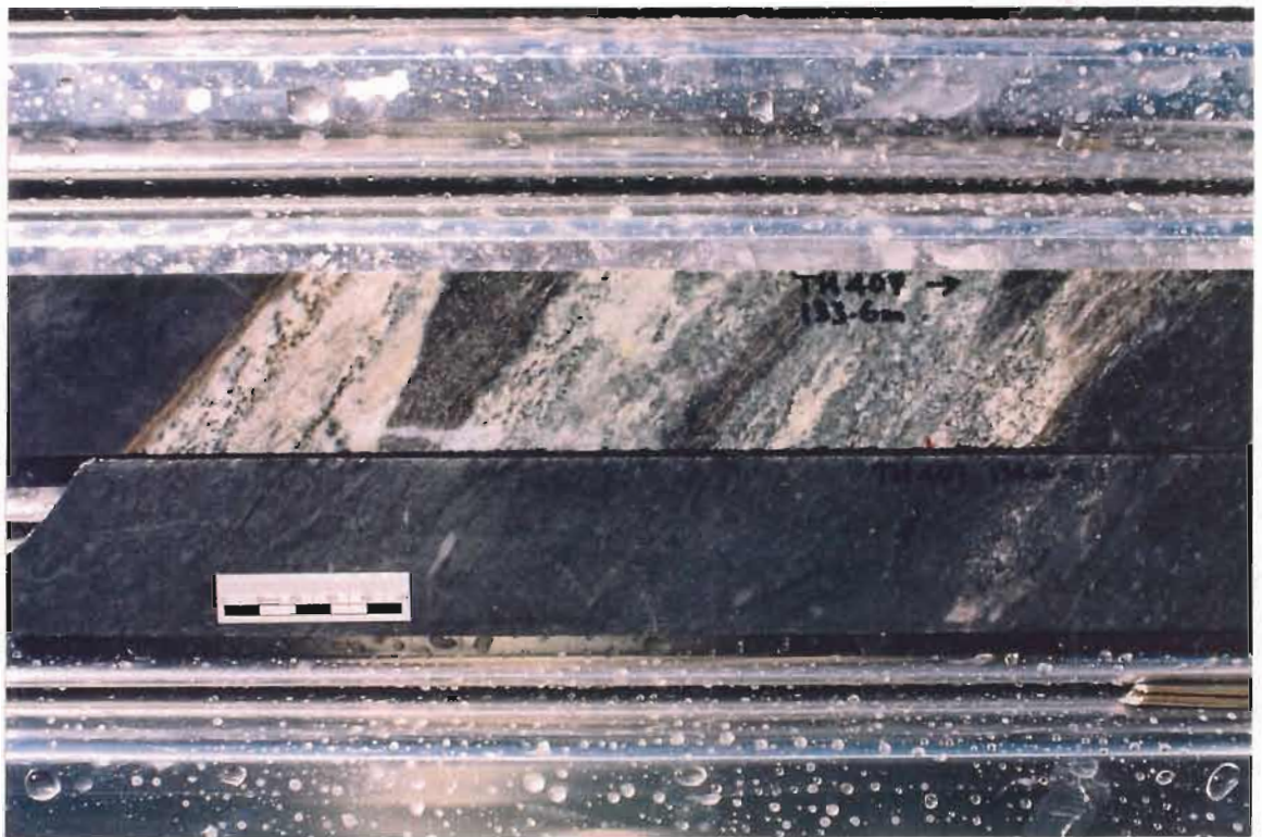
Figure 26. Band or patch of semi pervasive pale clinozoisite-carbonate and dark green actinolite alteration in otherwise weakly quartz-sericite altered footwall rhyolite; core from TH407, 133.6m, West Thalanga Extended.
