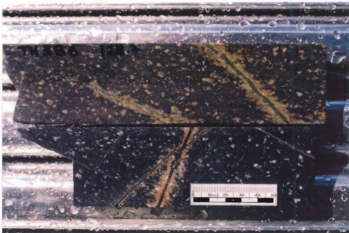
Figure 12a Sawn core specimens of porphyritic dacite showing vein epidote-albite alteration selvages with feathery margins suggesting alteration pervaded outwards along pre-existing weak S2 cleavage
