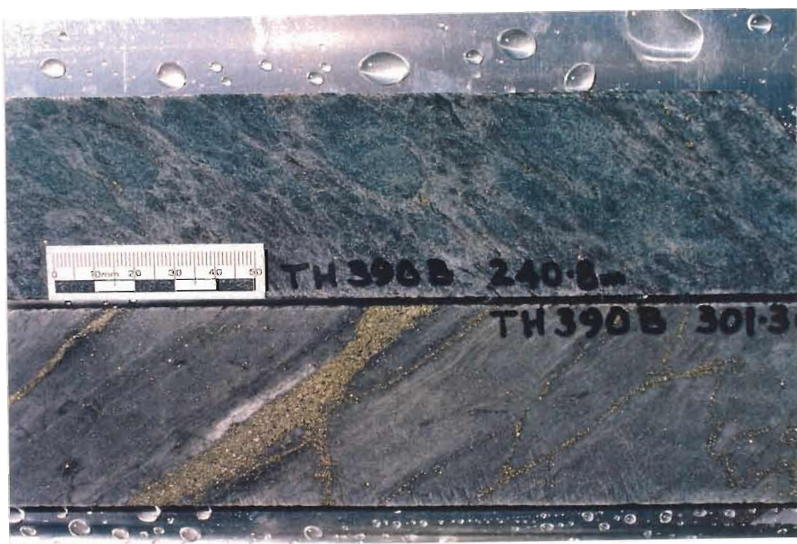
Figure 21. Upper specimen: blotchy chlorite fabric in moderately altered, formerly coherent? rhyolite typical of Group 2; very common in East Thalanga footwall. Lower specimen: intensely silicified, "de-textured" rhyolitic rock with pyritic stringers; characteristic of Group 4 in footwall stringer zone.
