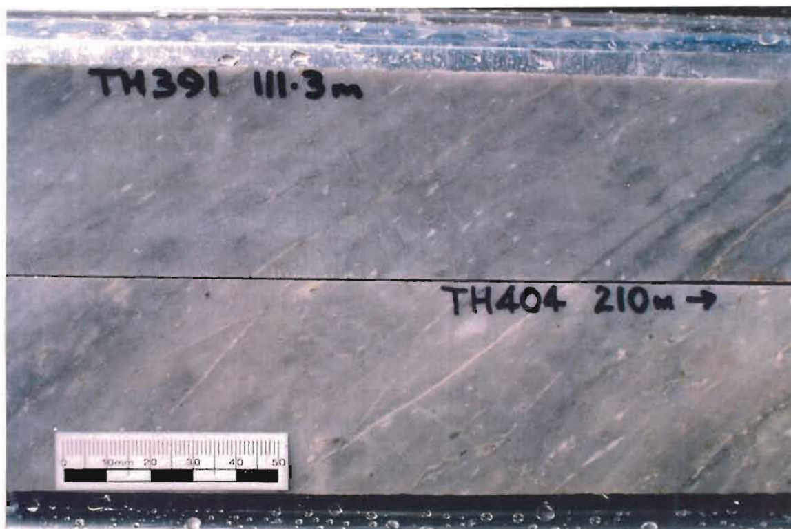
Figure 22. Sawn core specimens of silicified "white" rhyolite from footwall of East Thalanga area, exemplary of Group 5. Similar rocks occur in Central and West Thalanga footwall, sometimes well down in the stratigraphic sequence below the favourable horizon
