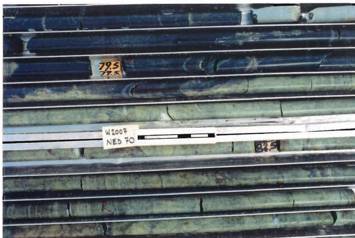
Figure 10b. Diamond drill core from W2007NED70 (before sawing of samples 60224 & 60225) showing strong, domainal, partly fracture controlled, epidote-quartz alteration in fresh dacite.
