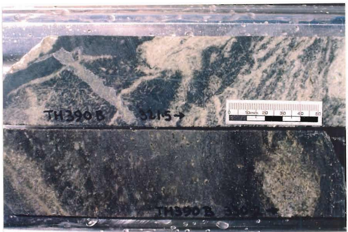
Figure 27. Core specimens from TH390B in footwall of East Thalanga deposit (Fig. 3 of text). Upper: massive felted chlorite (dark) with irregular bands of pale green-white tremolite. Lower: massive felted chlorite-phlogopite with scattered bunches of fibrous tremolite, gradational into relict rhyolite with incipient clinozoisite-actinolite alteration.
