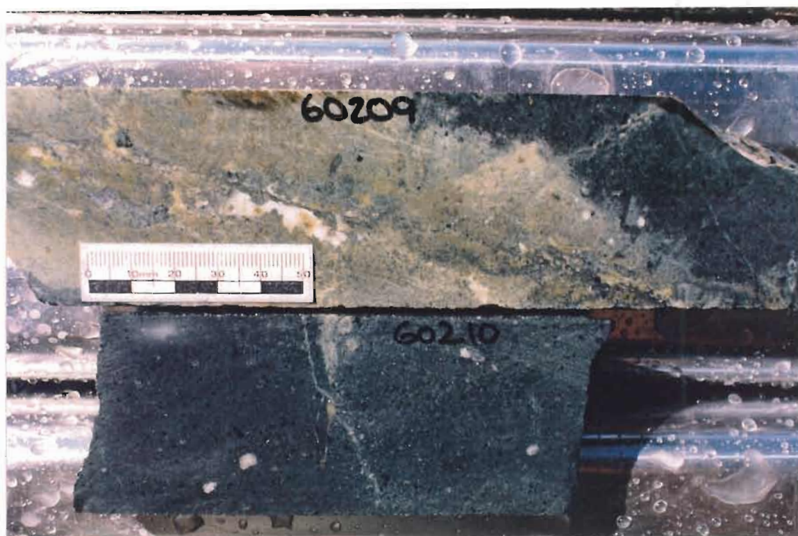
Figure 10a. Photograph of altered and unaltered "andesite" samples 60209 & 60210 from TH407 showing sharp boundary of pervasive epidote-albite-(carbonate-actinolite) alteration.
