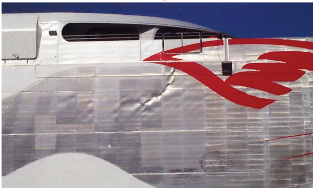
Figure 1.14: Side shell buckling as a consequence of severe slamming loads, Hull 50 of Incat Tasmania.
