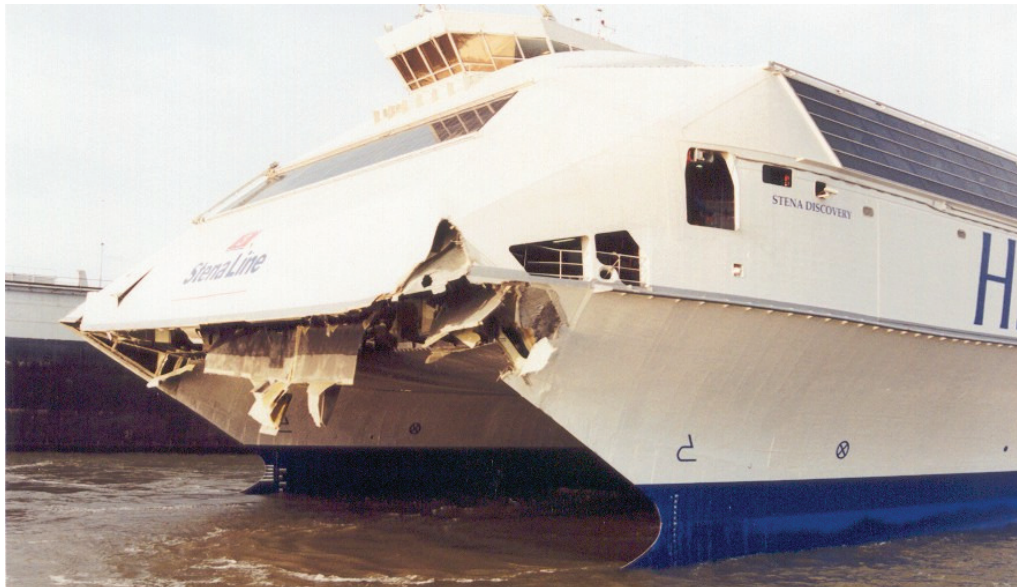
Figure 1.13: Damage of bow structure on HSS 1500 Stena due to severe slamming loads.
