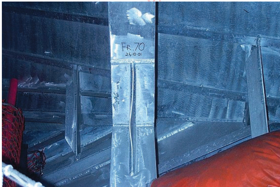
Figure 1.15: Tripping of brackets and vertical stiffeners in the centre bow of Hull 50 of Incat Tasmania due to severe slamming load.
