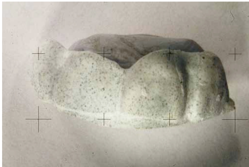
Figure 4.6. Epoxy resin replicas containing titanium oxide paint colourant and coloured particles. Image acquired with Lieca R5 Elcovision and macro lens, at a photoscale of \times 2 and swan halogen lighting.
