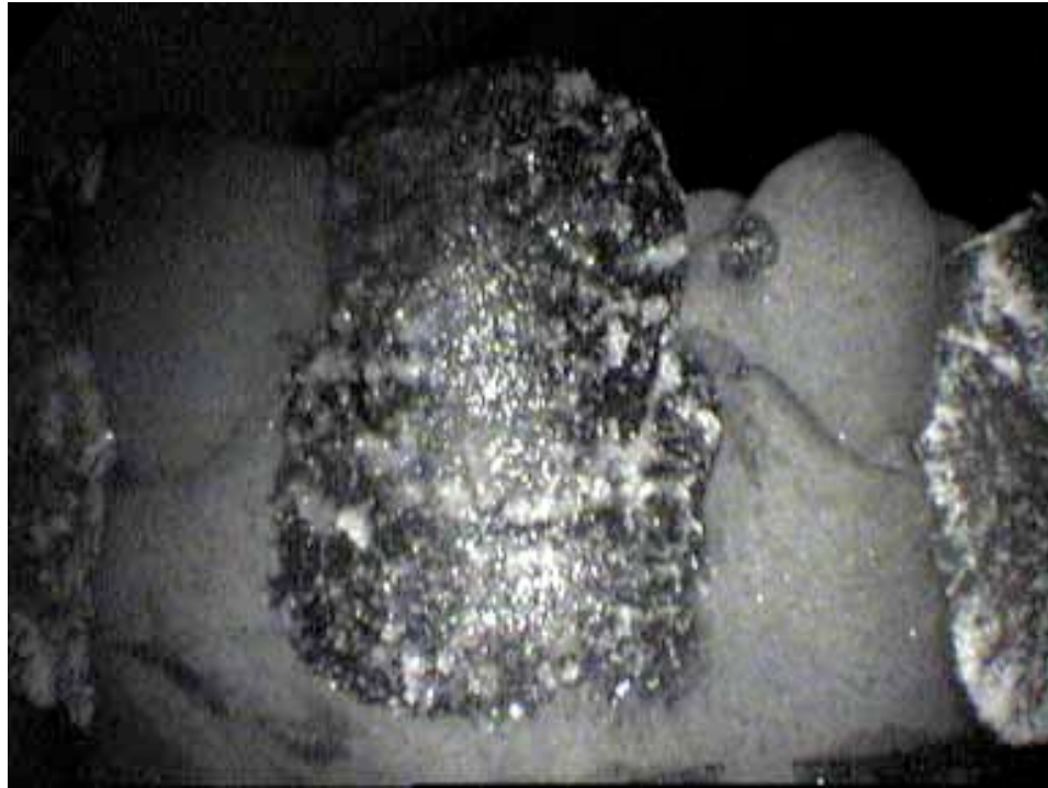
Figure 4.5. Plaster model, coloured with black pigment, enamel bonding resin, 50 µm aluminium oxide applied with air brush. Imaged with video otoscope (MAICO-Vision MV10; MAICO Diagnostics GmbH, Rohrdamn, Germany).
