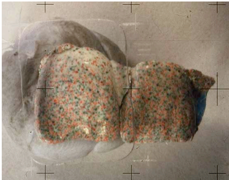
Figure 4.7. Epoxy resin replicas containing titanium oxide powder and coloured particles. Image taken with Lieca R5 Elcovision, 100mm macro lens, at a photoscale of x2 and swan halogen lighting.
