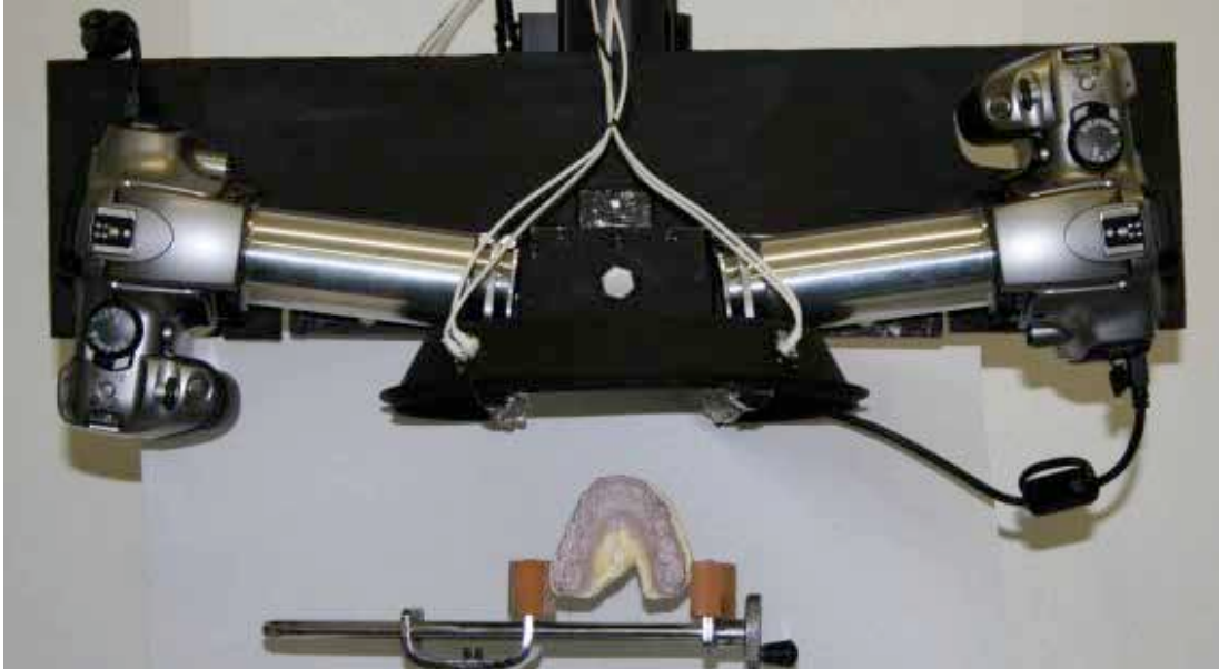
Figure 9.3. Fixed base stereo camera, lens and mirror assembly with LED illumination. (also refer to Figure 7.2, pp. 124)
