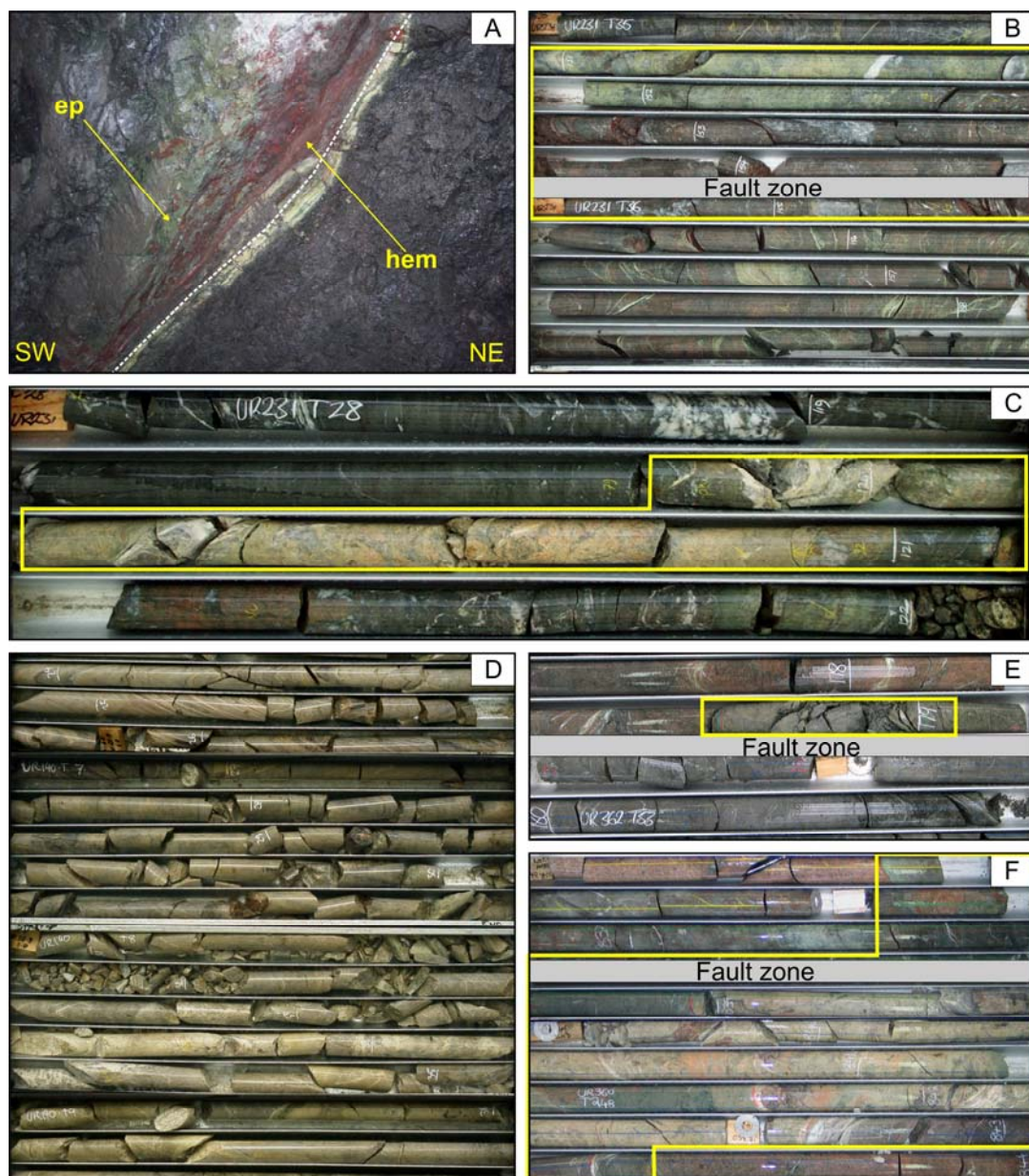
Figure 5.8 North-northwest striking low-angle thrust faults at Ridgeway. A) Purple Fault exposed underground (340/65°SW), comprise of 6 cm clay - epidote - hematite fault gouge with up to 30 cm epidote - hematite alteration halo from the contact (5100mRL-XC22-chainage 96). B) Drillcore intersections of Purple Fault zone (yellow box) characterized by a 3.5 m zone of pervasive epidote - hematite alteration (UR142-152-155.5m). C) Photograph of Rimmers Fault (yellow box) characterized by a 1 m pervasive quartz - carbonate alteration halo. The fault contact separates the pyroxene-phyrlic dike and volcanoclastic sandstone (UR231-120-121m). D) Drillcore intersection of the Allana Fault with an extensive quartz - carbonate alteration halo transected at 5100mRL (UR140-24-37m). E) Photograph of Claudia Fault (yellow box; UR362-178.7m). F) Photograph of Pamela Fault (yellow box; 050/10°NW), a 7.5 cm cemented fault breccia with epidote flooding. This fault marked the sharp contact of the late-stage quartz monzonite (hanging wall) and monzodiorite (footwall). Quartz - carbonate alteration haloes are well developed on the monzodiorite (UR360-836m). Abbreviations: ep = epidote, hem = hematite
