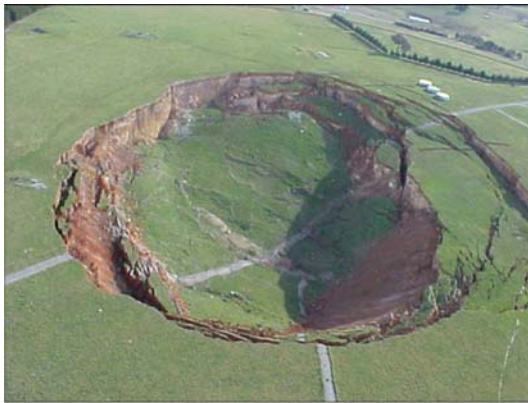
Figure 1.4 Aerial photo showing the subsidence zone on top of the Ridgeway mine, ca. 2003. Photo courtesy of Newcrest Mining Limited.
