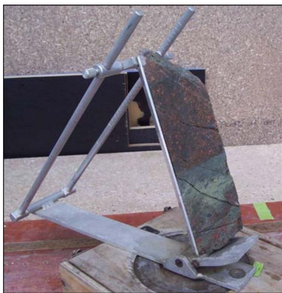
Figure 5.1 “Core-orientation cradle” used to measure the dip and dip direction of structures from oriented drillcores at Ridgeway.
