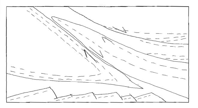
Figure 5.7: Representation of the planes of movement, and bedding orientations, within dextral shear zone developed in the Owen Conglomerate east of the Darwin Plateau. This shear zone is shown in Plate 5.2.
