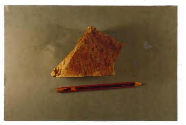
Plate 5.3: Mylonite. A zone of mylonite is developed in the equigranular granite at the northern end of the Darwin Plateau. Quartz occurs in elongate bands, feldspar porphyroclasts (rounded to fragmented) are rotated.
