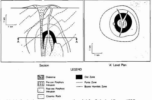
Figure 6.4: Model of a classic-type porphyry copper deposit (after Sutherland Brown, 1976).
