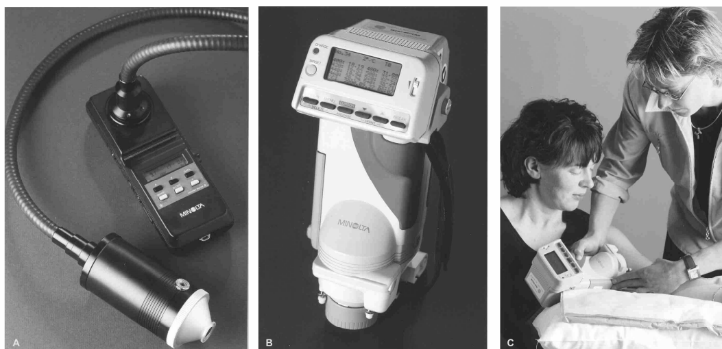
Figure 3. A chroma-meter (A) and spectrophotometer (B), used to estimate melanin density of the skin at a body site usually not exposed to the sun by measuring skin reflectance (C).
