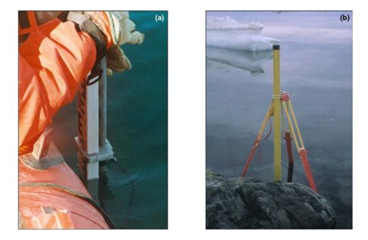
Figure 5-24 Datum connections to the submerged pressure gauges. (a) Direct measurement. (b) Timed water level measurements (Images courtesy of R. Handsworth).
