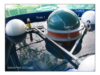
Figure 2-11 GPS Buoy in deployment configuration in a saline pool. Note the position of the three scales.
