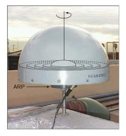
Figure 2-13 SCIGN short dome shown with the choke ring antenna surface superimposed over the dome. The section below the top of the choke ring is cylindrical, the section above is hemispherical. (Photograph from Hudnut, 1999).
