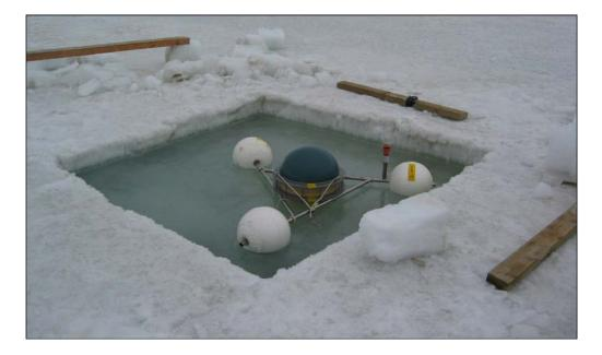
Figure 5-25 GPS buoy over the Davis bottom mounted pressure gauge.
