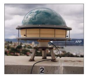
Figure 2-15 The GPS dome apparatus attached to the Leica AT504 antenna on Pillar
