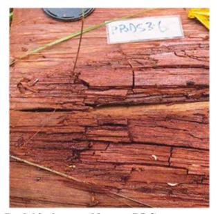
**Dark blocky crumbly rot - DBC** Dark blocky crumbly rot is characterised by brittle wood that breaks off in regular blocks and can be crumbled to powder by hand. It is tan or light brown in colour and contains consistently contains very dry sheets of mycelium, with a chamoislike texture that progress along the rays.
