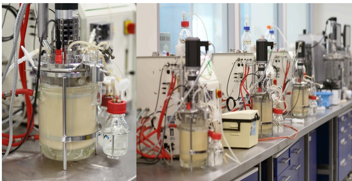
Figure 5-1 Two litres stirred tank bioreactors connected to a Biostat B (Sartorius Stedim, Australia) control system
