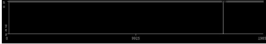
Fig. 2. The classification diagram produced by the SVM. The X-axis is the position within the input sequence data. The top line represents the locations of negative predictions. Notice the clear gap in negative predictions centred on the TSS position (indicated by the white line)
