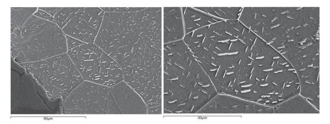
**Figure 7.** SEM image of the iberian pilum, a massive iron carbide precipitate in a ferrite grain matriz with Widmannstätten type structure can be seen (7 a left)); detail from Fig. 7 a); idiomorphic iron carbide morphology and presence of cementite at the ferrite grain boundaries can be distinguished (7 b right)).
