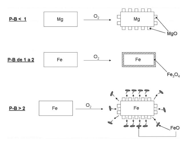
**Figure 5.** Scheme relating the formation of different oxides with its corrosion protector behaviour as the ratio Pilling-Bedworth classifies them.
