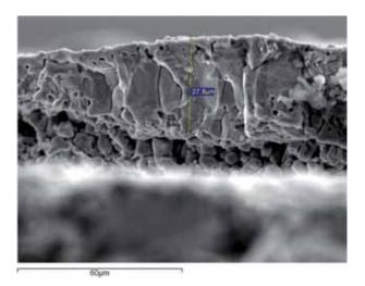
**Figure 12.** SEM image of the artificially created magnetite layer. The furnace was operated under oxidising atmosphere over 10 min applying boron oxide as fluxard.
