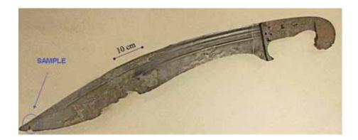
**Figure 1.** Iberian falcate, belonging to the collection of the Museum of Armory in Vitoria, Álava. The site where the sample was extracted is highlighted.
