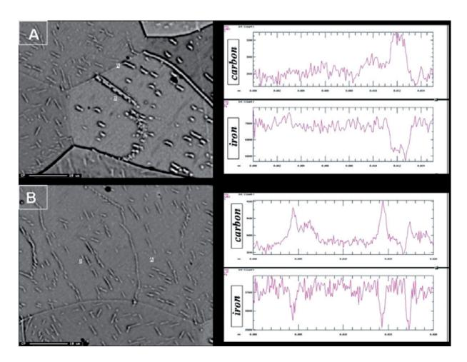
**Figure 9.** SEM images and corresponding results of EPMA. The fact that the analytical profile shows an increase of carbon combined with a decrease of iron when analyse the crystals with Widmannstätten structure indicates presence of iron carbide. The upper image corresponds to the pilum and the downer to the falcata.
