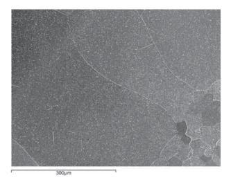
**Figure 11.** SEM image of the falcata sample. The elevated grain size in the outer zone versus the small grains in the interior can be clearly distinguished.
