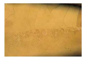
**Figure 10.** Image of a cross section of the falcata sample obtained by optical microscopy. The elevated grain size in the outer zone versus the small grains in the interior can be clearly distinguished.
