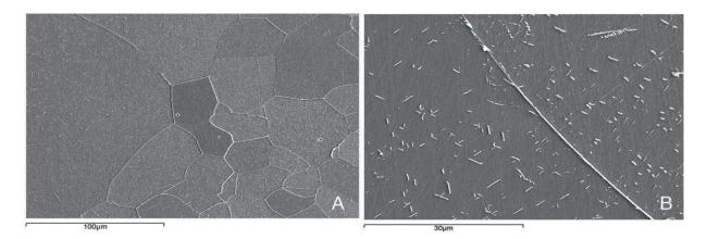
**Figure 8.** The structure of the metallic core of the falcata. A fine grained precipitate of iron carbide in a ferritic matrix of varying particle size is shown (Fig. 8 a)); detail from Fig. 8 a), idiomorphic iron carbide with Widmannstätten structure in the interior of ferrite grains are shown, as well as continuous cementite precipitation at the grain boundary (Fig. 8 b)).
