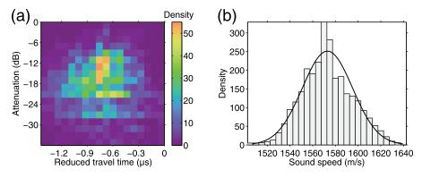
Fig. 2. (Color online) (a) A two-dimensional histogram of relative attenuation vs reduced travel time data. (b) Histogram of sound speed calculated by Eq. (1). The mean 1573.0 m s<sup>-1</sup> and SD 22.2 m s<sup>-1</sup> of the fitted normal density (solid line) provide an estimate of average tissue sound speed of the E. radiata sample.
