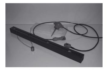
**Fig. 1.** A georod prior to epoxying the geophone elements into the wells, along with a conventional 28 Hz geophone. A 40 Hz geophone element (left) is inserted into each of the wells within the georod body and connected in series. Both the georods and conventional geophones are fitted with split-plate connectors for coupling to the seismic cable.
