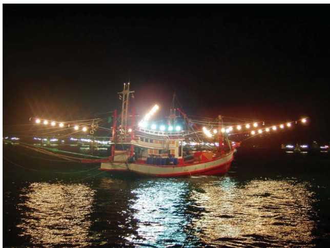
Figure 48. A falling net boat participating in squid light luring fishery for loliginid squid in Thailand.
