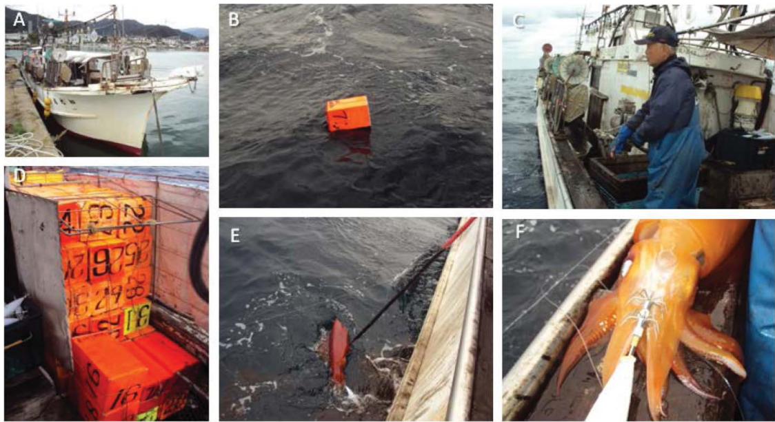
Figure 76. Photos showing how Thysanoteuthis rhombus is typically fished in Hyogo Prefecture (Sea of Japan). (A) A typical boat used in the fishery. Most boats are operated by one fisher. (B) A bouy (float) resting on its side, indicating that no squid has grabbed a jig attached to the line. If a squid grabs a jig, the buoy will stand up. (C) When a fisher spots a standing buoy, the gear is retrieved using a winch and by hand. (D) Buoys on deck. (E) When the squid reaches the surface, it is gaffed or netted, and brought onboard (F).
