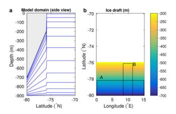
**Fig. 1.** Model geometry from (a) side view, with bathymetry at 900 m below the surface and ice shelf shown in grey and every second sigma level shown in blue. (b) Ice shelf linearly slopes down to 700 m with a 200 m thick ice front at 76°S. Location of zones averaged for Fig. 3 are marked A and B.
