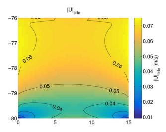
**Fig. 6.** The depth-averaged RMS tidal velocity for the zero forcing + tide run, showing strongest currents across the middle of the ice shelf. The currents are temporally-averaged across an integer number of tidal cycles.
