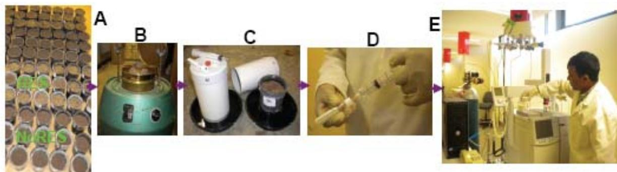
**Figure 1.** Summary of the methodology: (A) treatments prepared, (B)  $< 4\text{ mm}</math> sieve mounted on sieve-shaker to simulate tillage, (C) sealed chamber used for headspace gas sampling, (D) samples in evacuated vials and (E) sample analysis by gas chromatograph.$
