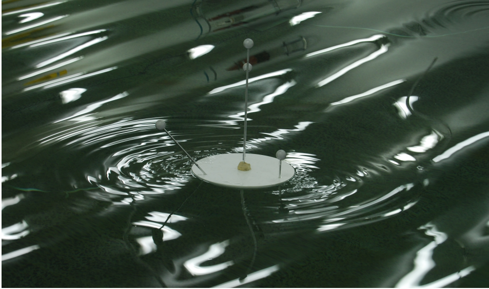
Figure 2: Model floe during test. Scattered waves are evident.
