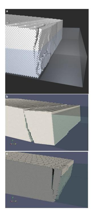
**Fig. 3.** Contrasting calving styles modelled in HiDEM. (a) Ice-cliff failure modelled using  $D_{\rm W}/D_{\rm F}=0.61$  and  $U_{\rm L}=0$ . The subaerial ice face is 44 m high. (b) Buoyancy-driven calving with  $D_{\rm W}/D_{\rm F}=1.1$ ,  $U_{\rm L}=0$ , showing upward growth of basal fracture and block rotation. (c) Melt-undercut calving with  $D_{\rm W}/D_{\rm F}=0.9$ ,  $U_{\rm L}=20$ .
