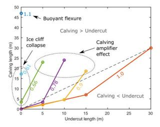
**Fig. 4.** HiDEM calving lengths as a function of undercut length for different relative buoyancies ( $D_{\rm W}/D_{\rm F}=0.61$ , 0.66, 0.78, 0.9, 1.0 and 1.1). The lines are intended to aid visual grouping of results, and do not imply linear variation between plotted points. Each set of connected points represents one row on **Figure 2**, and can be viewed as an evolutionary sequence. For each value of relative buoyancy, increasing the undercut length produces larger calving events.
