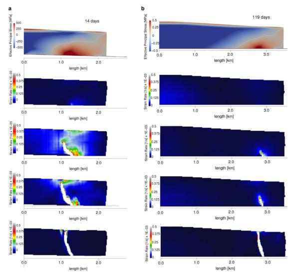
**Fig. 7.** Modelled calving events for (a) the sloping bed case at t = 14 days; and (b) the horizontal bed case at t = 119 days. Top panel: effective principal stress in Elmer/Ice; Lower panels: snapshots of the HiDEM simulations, showing strain rates in inter-particle beams averaged through the width of the model domain. The averaging creates a false impression of a wide crack: fracture geometry is shown in Figure 8.
