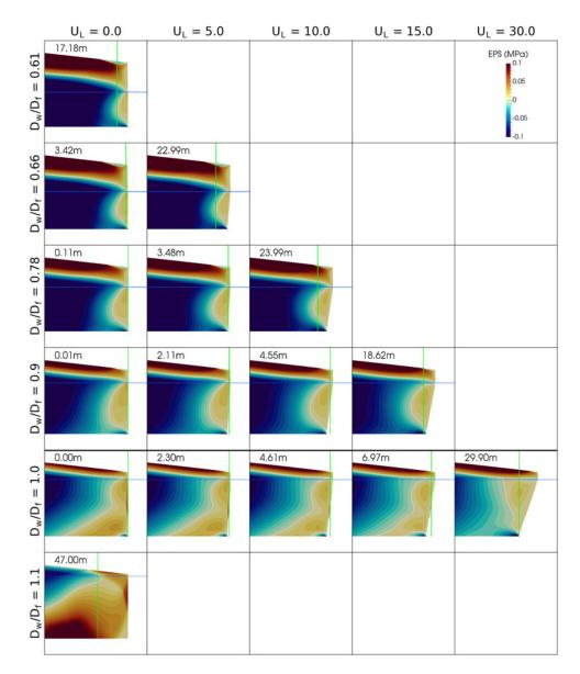
**Fig. 2.** Matrix of ice-front geometries used in the melt-under-cutting experiments, showing Effective Principal Stresses (EPS calculated in Elmer/Ice and HiDEM calving length indices (vertical green lines and figures in each panel).
