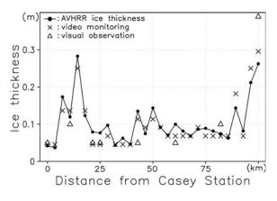
**Fig. 5.** Comparison of sea-ice thickness derived from the three methods along the cruise track in the Vincennes Bay polynya during the daytime, with the abscissa being the distance from Casey Station.
