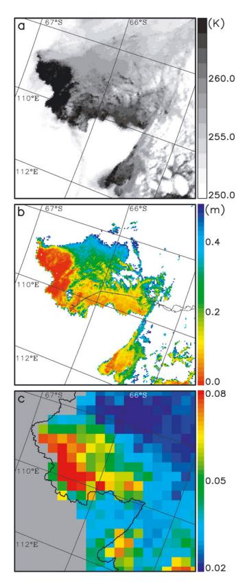
**Fig. 2.** Comparison of the AVHRR and SSM/I imagery for the Vincennes Bay region of East Antarctica on 19 October 2003. Maps of (a) the AVHRR ice-surface temperature; (b) the AVHRR ice thickness with the cruise track superimposed; and (c) the SSM/I polarization ratio at 85 GHz ( $PR_{85}$ ) with the ice-shelf edge inferred from the AVHRR data superimposed. The white pixels in (b) show an area of thick ice with thicknesses of >0.5 m including ice shelf and continental ice sheet.
