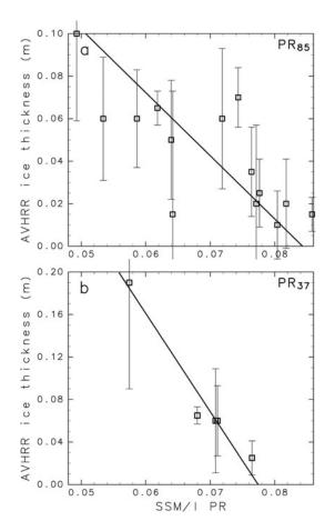
**Fig. 6.** Scatter plot of the AVHRR ice thickness vs SSM/I PR for (a) 85 GHz and (b) 37 GHz. The solid line denotes the principalcomponent axis of these plots. The vertical lines with crossbars show the standard deviation of AVHRR ice thicknesses in the SSM/I gridcell in each plot.
