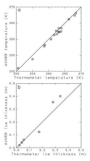
**Fig. 3.** Scatter plots of (a) the AVHRR temperature vs thermometer temperature; and (b) the AVHRR ice thickness vs the thermometer ice thickness.
