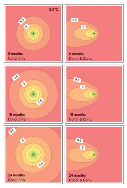
**Figure 4.** Heat flow profiles at various time steps (water flow velocity: (0.16 m/day); the temperature difference between each iso-counter line is  $(0.5^{\circ}\text{C})$  and the numbers in the white text boxes refer to the temperature of the respective iso-counter lines, in  $^{\circ}\text{C}$ ).
