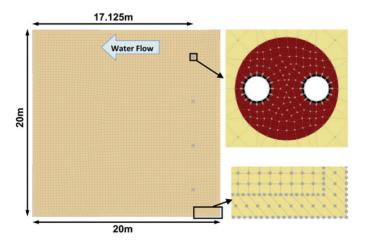
Figure 2. Soil cluster with multi-boreholes.
