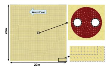
Figure 1. Soil cluster with centralized borehole.
