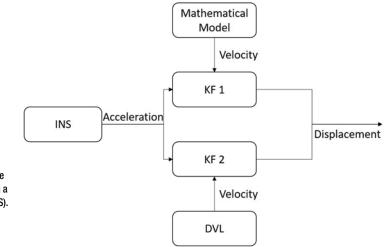
Figure 1: The block diagram of an overall process for model-aided INS localization. Once INS measures acceleration data from AUVs' trials, the data are combined and amended with a mathematical model using KF (MA-INS). INS data are also combined with DVL result by another KF, and the data are applied to MA-INS intermittently.
