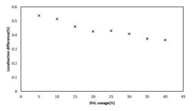
Figure 8: The localization percent difference comparison of MA-INS localization solution with various DVL uses in 20 second regular intervals. The percent difference is decreased when DVL usages is longer, but only 0.37% of percent difference was decreased between 1 second and 8 seconds.
