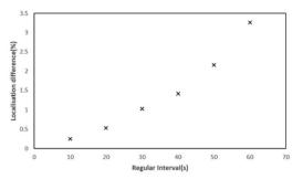
Figure 9: The localization percent differences of MA-INS localization solution with various DVL uses in a 20 seconds regular interval. As the interval of DVL operation is increased to 60 seconds, the percent difference increases to 3.5%.
