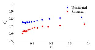
Figure 8. Variation of contraction constant,  $C_c$  with with K at h/d = 0.1 for nozzle 6 with water saturated at the supply pressure and with unsaturated water (atmospheric pressure) assuming choked flow conditions as per equation 1.
