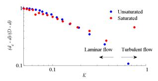
Figure 7. Variation of cavity diameter with *K* at h/d = 0.1 for nozzle 6 with water saturated at the supply pressure and with unsaturated water (atmospheric pressure) at showing regions of laminar flow and where the cavities destabilise to turbulence and microbubble generation.
