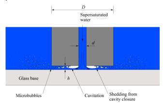
Figure 1. Schematic of the experimental setup showing the confined radial jet formed between the inlet nozzle and a glass wall permitting visualisation of the cavitation occurrence.
