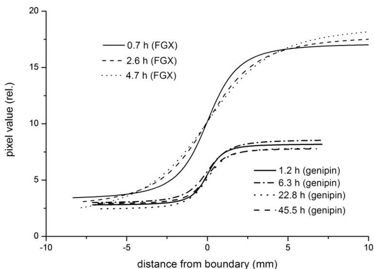
**Figure 1.** Fitted curves of image profiles of FGX gel (upper curves) and genipin-gelatin gel (lower curves) obtained at various times.
