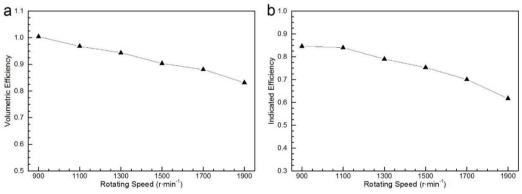
Fig. 3. (a) volumetric efficiency varying with rotational speed; (b) indicated efficiency varying with rotational speed.
