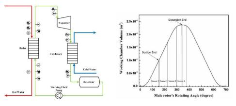
Fig. 1. (a) Schematic drawing of the ORC system test rig;
