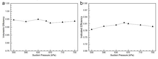
Fig. 4. (a) volumetric efficiency varying with suction pressure; (b) indicated efficiency varying with suction pressure.
