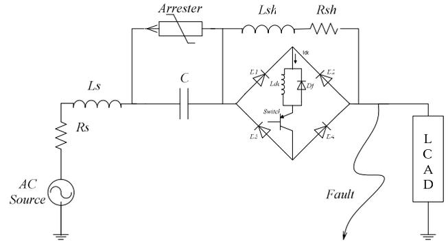
Fig. 2. Power system with the proposed FCL
