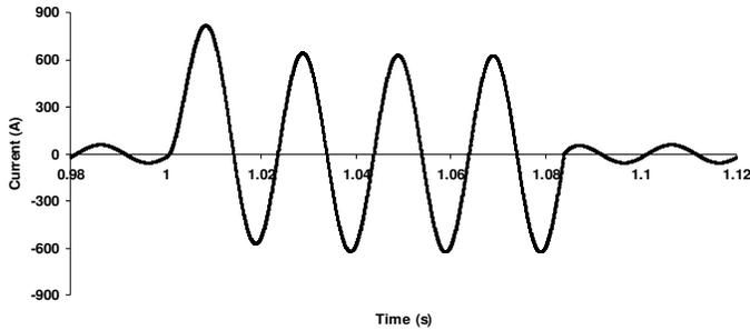
Fig. 4. Line current without the proposed FCL
