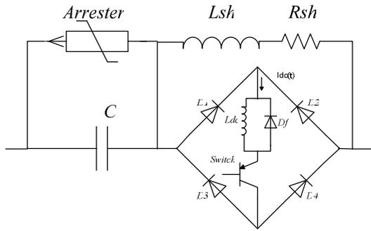
Fig. 1. Power circuit topology of the proposed FCL
