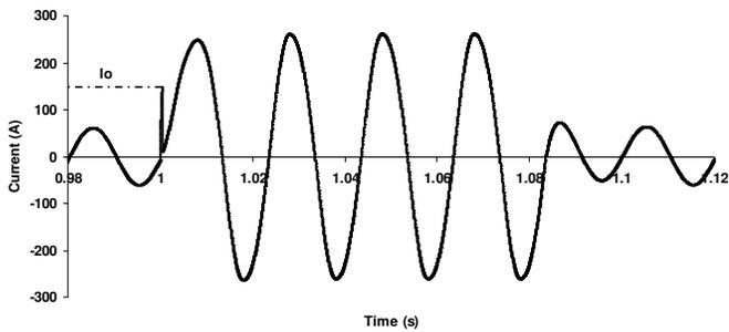
Fig. 5. Line current with the proposed FCL
