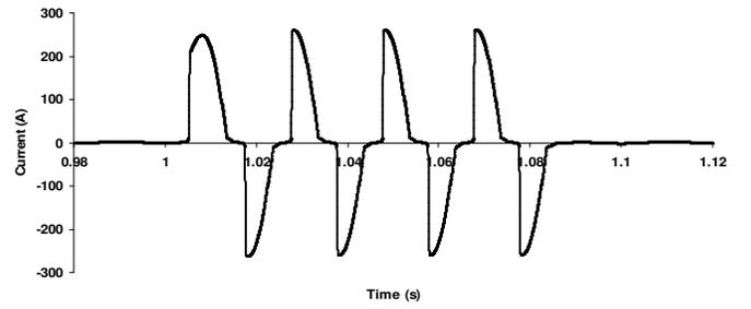
Fig. 6. Arrester current
