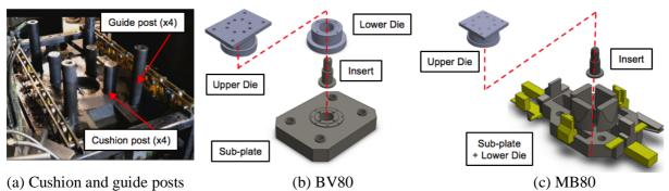
Figure 1. Components in the machine and dies set [5]
