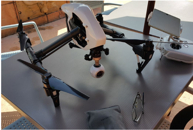
Fig. 13. 360 camera retro fitted on a drone.
