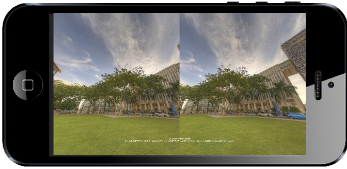
Fig. 5. Stereo viewing mode adaptable for mobile-based HMD.
