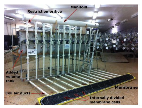
**Figure 3** A photograph of the experimental set-up for the Bombora WEC model (while the basin was drained). The flexible membrane is the black material in the foreground. The pipework behind the WEC model provided a means of measuring air flows and pressures in the system (and to correctly scale the required air volumes) [1].
