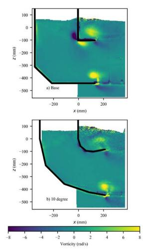
**Figure 4** PIV results showing the average vorticity (energy losses) within two different OWC geometries. The significant reduction in losses around the upper lip is evident between the base geometry (top) and the smoother transition of the 10 degree lip case (bottom). The PIV data can also be used to examine the average kinetic energy of the velocity fields which can identify inefficiencies as an uneven distribution is likely to result in further energy loss [8].
