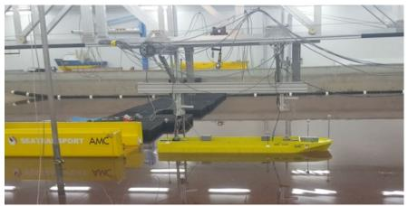
**Figure 5** Photograph showing the scale model of the feeder vessel (right) about to travel astern to enter the stern well dock of the FHT (left). In addition to acquiring PIV data of the complex flow inside the well dock as the feeder performs this manoeuver, the dynamic effects on the hull resistance (powering) and motions were also quantified.
