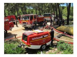
**Re-supplying a whole strike team at once**. The French have a specialist water supply function which is capable of resupplying a whole strike team at once in about 6 minutes. The set-up consists of a large capacity bladder tank or fixed water supply tank, a large capacity volume pump and a manifold which allows all 4 appliances to be filled at once. This makes the re-supply of strike teams very efficient.
