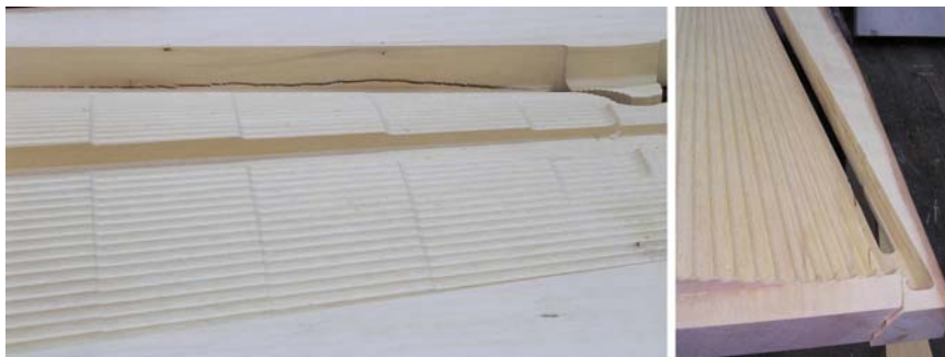
Fig. 3: From left to right; a longitudinal crack caused by letting the router bit run diagonally against a long grain of wood (Kongsuwan 2011)
