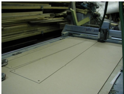
Fig. 10: While 9 mm of MDF was cutting by CNC in order to produce the shelves' template. (Kongsuwan 2009)
