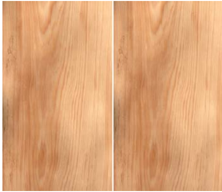
Fig. 14: The feature of sequential or slip matched veneer (Kongsuwan 2009)
