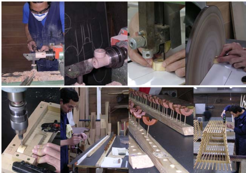
Fig. 73: From left to right; the sequence of stages in executing and assembling the feet of the Dowel Bench Seats, made of horizontal scrub timber (Kongsuwan 2010)
