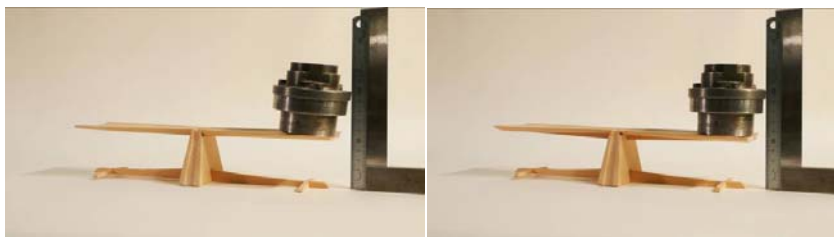
Fig. 12: From left to right; the stable test of Cantilever Bench #3 and #4's scaled models (Kongsuwan 2009)
