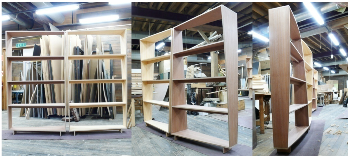
Fig. 56: The second assembly of a pair of Trapezoidal and Curvilinear Shelves shows tapering and curved edge of underneath beams. (Kongsuwan 2010)
