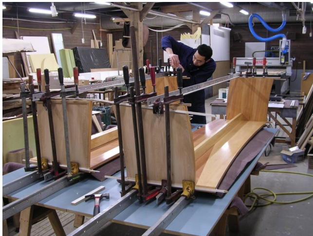
Fig. 7: The processes of joining and gluing horizontal and vertical boards (Kongsuwan 2010)
