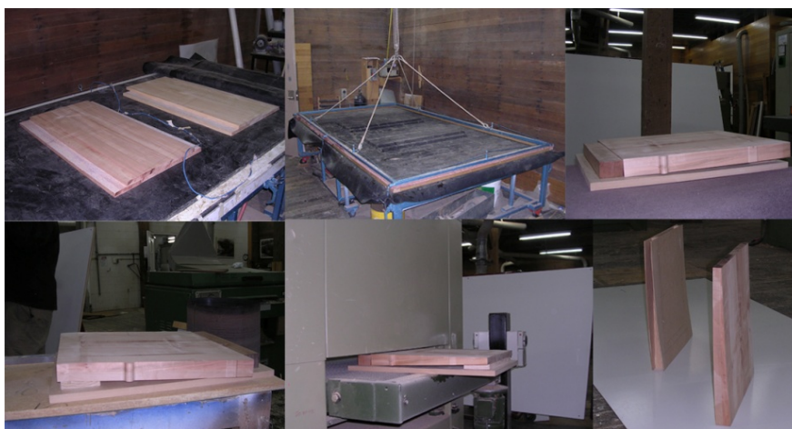
Fig. 6: The processes of subduing the stiff appearance of bench's legs (Kongsuwan 2009)
