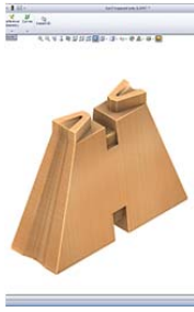
Fig. 17: The trapezoidal column of Cantilever Bench #5, rendered by Solid Works' software (Visalvate 2011)
