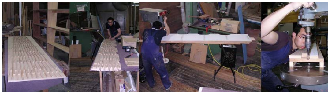
Fig. 21: Various jigs were developed for achieving an accurate drill (Kongsuwan 2010)
