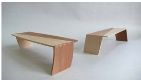
Fig. 38: From left to right; Diagonal Bench 2 was joined by common dovetails; and Diagonal Bench 1 was joined by a mitre joint. (Kongsuwan 2008)
