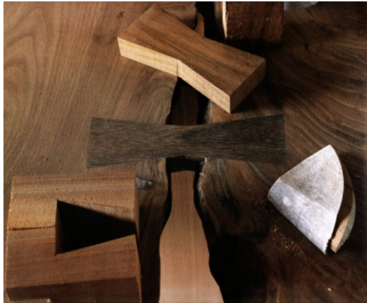
Fig. 23: butterfly keys and joints (Nakashima 2003, p.2)
