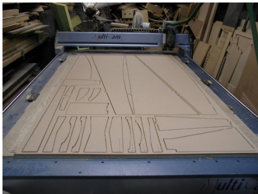
Fig. 40: The templates of Diagonal Benches while being cut by CNC router (Kongsuwan 2009)
