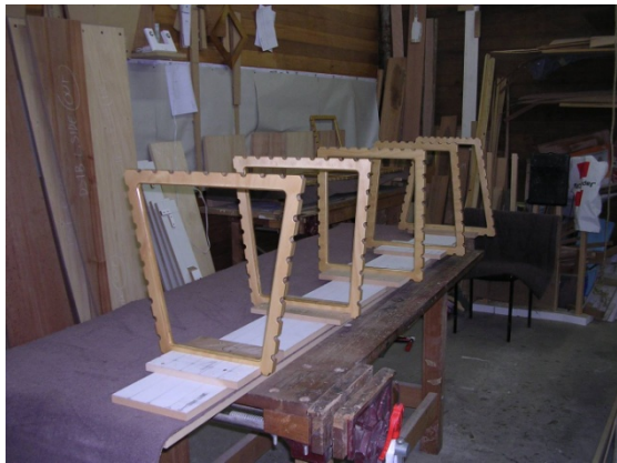
Fig. 27: Five vertical frames were arranged in place by a special jig. (Kongsuwan 2010)
