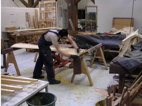
Fig. 4: Shaving the convex profile underneath a butterfly-shaped platform (Kongsuwan 2012)
