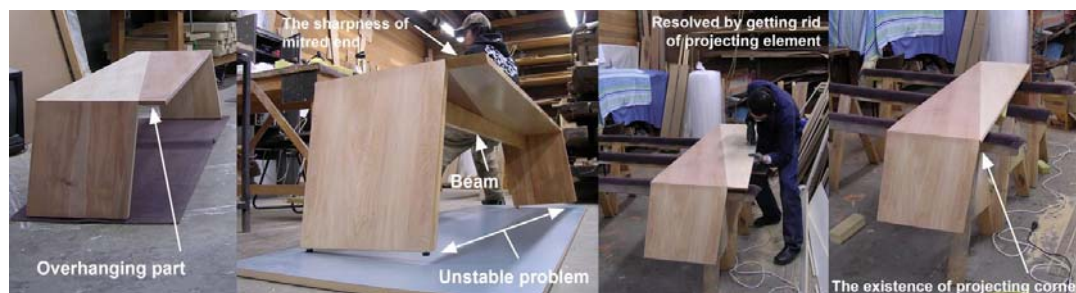
Fig. 41: The revision of Diagonal Bench 1 for greater stability (Kongsuwan 2010)
