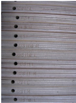
Fig. 17: Inscriptions were made by punching before the process of sanding, oiling and waxing. (Kongsuwan 2009)
