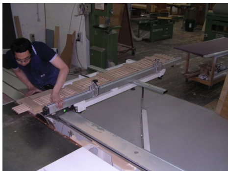
Fig. 22: A special jig was used to hold a set of dowels during the process of cutting. (Kongsuwan 2010)
