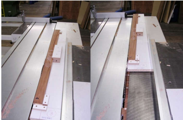
Fig. 55: Tapering one edge of rectangular beam by table saw (Kongsuwan 2009)
