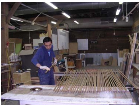
Fig. 24: Each length of dowel was hand-oiled. (Kongsuwan 2010)
