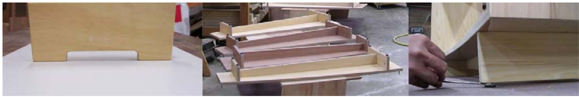
Fig. 57: From left to right; the first version of foot base; the feature of I-shaped base; and the demonstration of adjusting the feet (Kongsuwan 2010)
