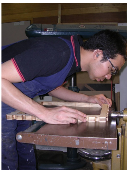
Fig. 26: While pre-drilling holes at frame's edge (Kongsuwan 2010)
