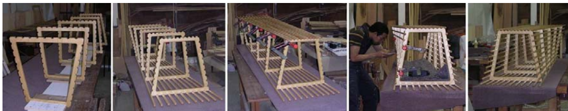
Fig. 75: The sequence of stages in assembling all linear components with five vertical frames (Kongsuwan 2010)
