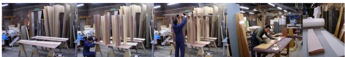
Fig. 67: The sequence of stages in the shelves' assembly and packing (Kongsuwan 2010)
