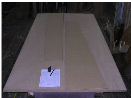
Fig. 11: Each template was used during the process of marking the outline of each component on plywood. (Kongsuwan 2009)
