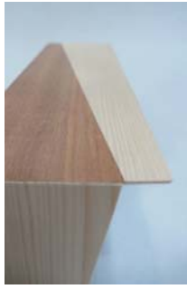
Fig. 35: The lineate conflict between a longitudinal grain of wood and a diagonal glued line (Kongsuwan 2008)
