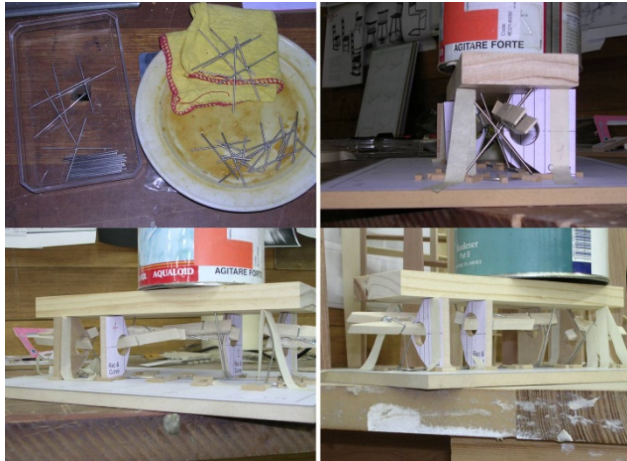
Fig. 30: Small jigs were used to achieve the precision of making miniature models. (Kongsuwan 2008)
