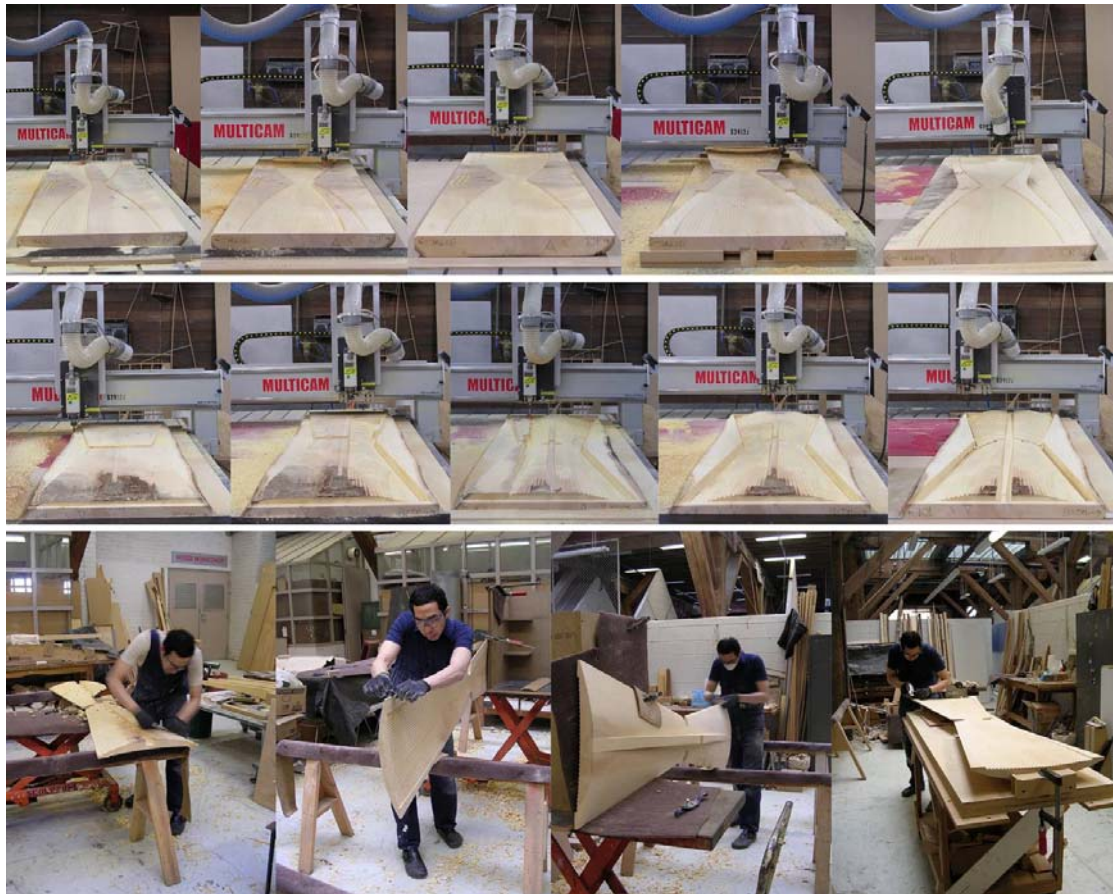
Fig. 31: From top to bottom row; the combination of digital technology and hands-on execution The first row; from left to right shows the processes of fluting and sloping the top surface of the seating platform. The second row; from left to right shows the sequence of stages in routing the bottom surface of the seating platform. The third row; from left to right depicts the processes of using hand-tools to enhance the sense of fluidity and the quality of the wooden surface. (Kongsuwan 2011)
