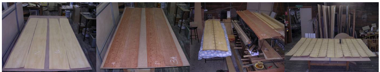
Fig. 15: The processes of book-matching and patching veneer (Kongsuwan 2009)
