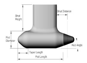
Figure 1. Geometric parameters used to define podstrut geometry.
