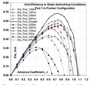
Figure 17. Unit efficiency plots for Pod 1 at different azimuth conditions.
