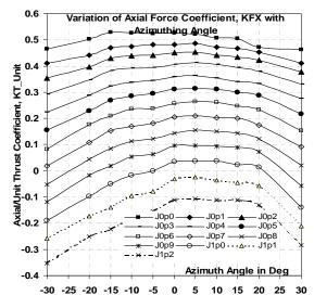
14(a) Unit Thrust / Longitudinal force coefficient
