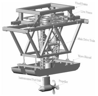
(a) the pod dynamometer system [10].
