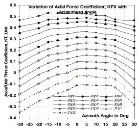
Figure 20(a). Unit thrust / Longitudinal force coefficient
