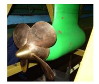
(e) propeller and the pod encasing the pod dynamometer
