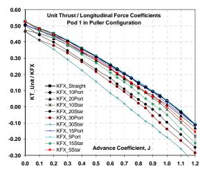
Figure 10. Longitudinal force coefficient plots for Pod 1 at different azimuth conditions.
