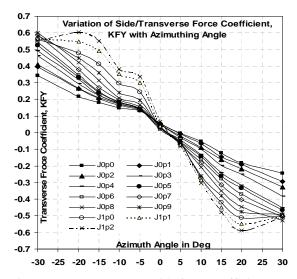
Figure 20(c). Transverse / Side force coefficient
