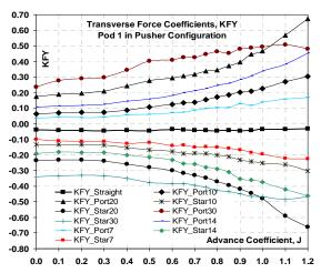
Figure 18. Transverse force coefficient plots for Pod 1 at different azimuth conditions.
