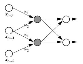
Figure 2. Time Delay Neural Network. In this example each hidden node only sees two time frames and weights are shared.
