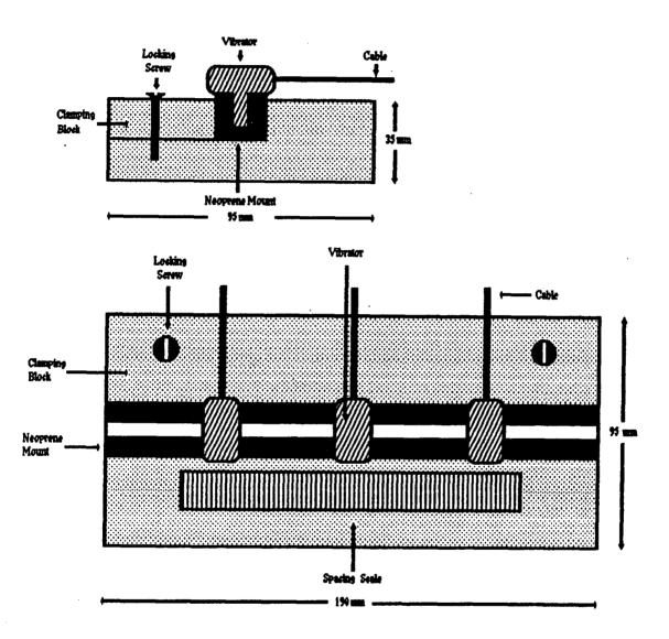
Figure 6.1: Schematic representation of the vibrator mounting device used in Experiment 7.
