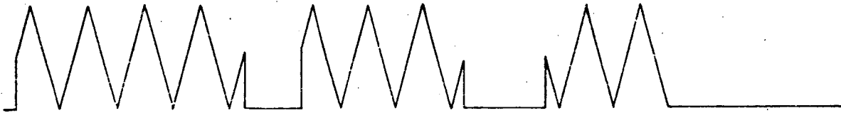
Modified Pulse width Modulation
