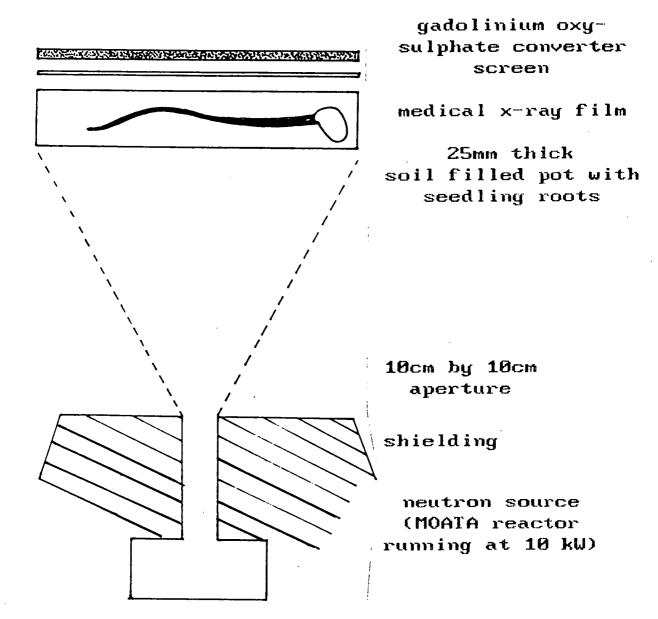
run. Single emulsion medical X-ray film (Kodak Lanex) was used for all experiments. The film was developed using Kodak D76 developer and an 8 minute developing time. Contact prints were made directly from the negatives, therefore figures are actual size.
