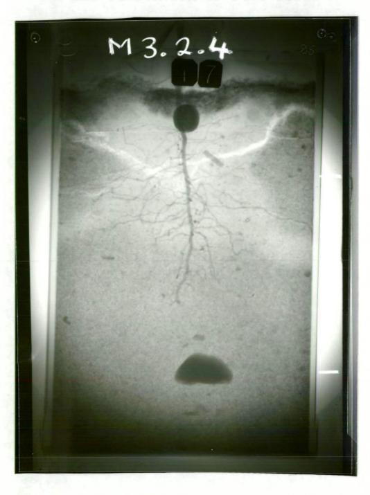
contents of 9% ( $\underline{c}$ . -30kPa) when determining the possible resolution of soybean roots possible. They inserted a cadmium strip bored with fine holes of varying diameters into the soil and observed that resolution of a hole of 0.33mm diameter was possible.
