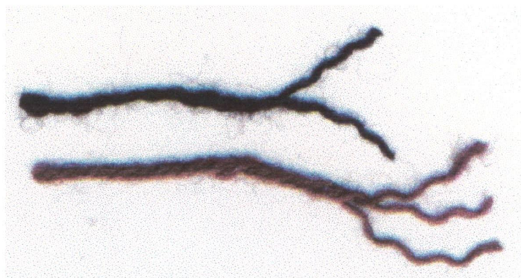
Figure 48. Navy two-ply yarn and mauve three-ply yarn
