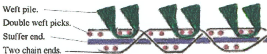
Figure 47. Detail, Axminster carpet construction
