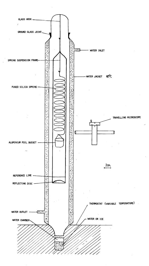
thin reference line mounted on the spring suspension frame (see figure 3.)
